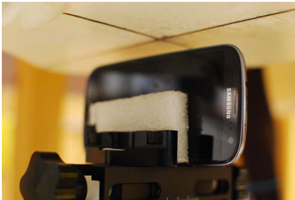
SAR Test Setup Photo 10: Left at 1.0 cm
