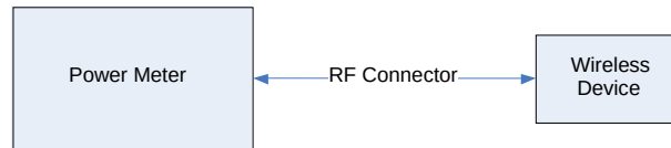
Figure 8-3 Power Measurement Setup
