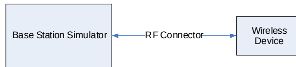
Figure 8-1 Power Measurement Setup
