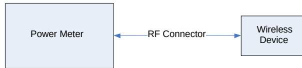
Figure 8-3 Power Measurement Setup
