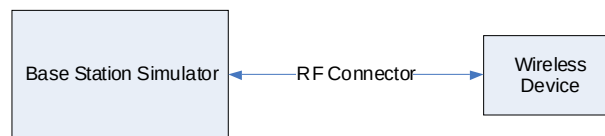
Figure 8-1 Power Measurement Setup
