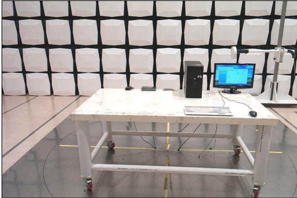
[ Radiated Disturbance for Below 1 GHz – Front ]
