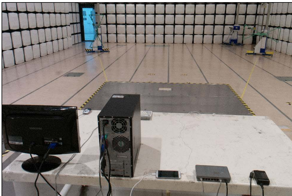
[ Radiated Disturbance for Below 1 GHz – Rear ]
