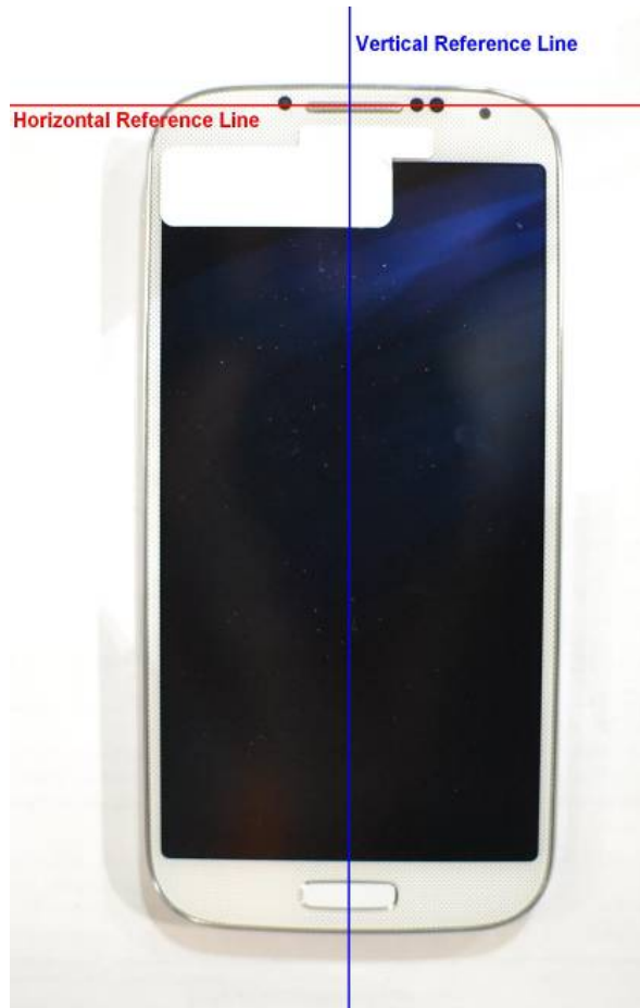
SAR Test Setup Photo 11 – DUT Reference lines
