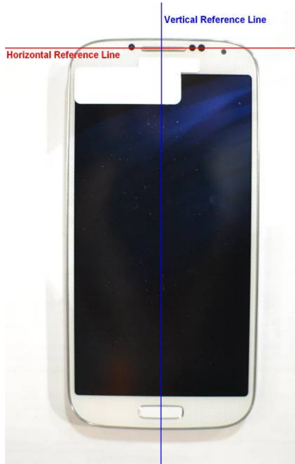
SAR Test Setup Photo 11 – DUT Reference lines
