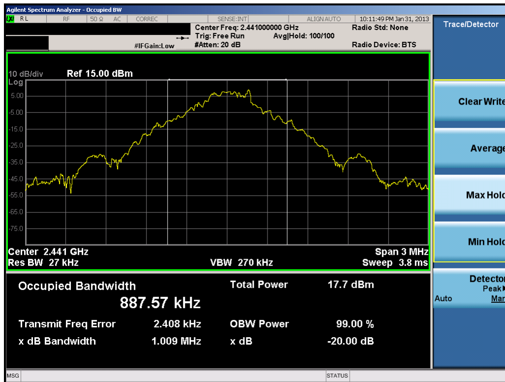
Plot 6-2. 20dB Bandwidth Plot (Bluetooth, 1Mbps – Ch. 39)
