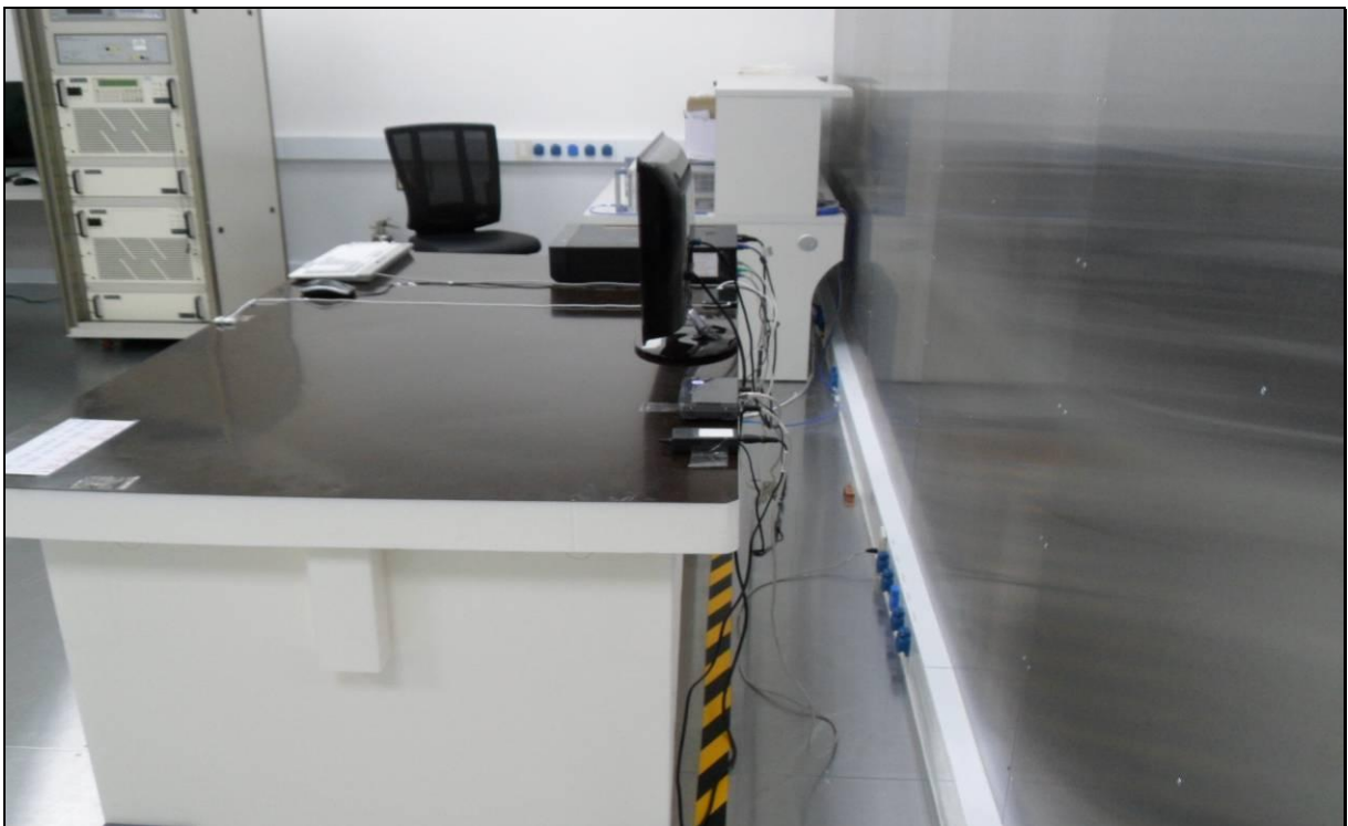
[ Conducted Disturbance – Rear ]
