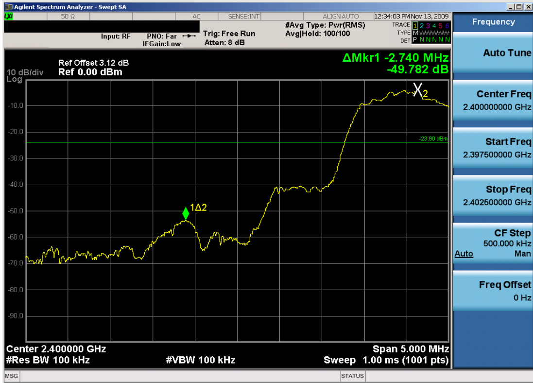
Plot 6-6. Band Edge Plot (Bluetooth 2.0 with Enhanced Data Rates – Ch. 0)
