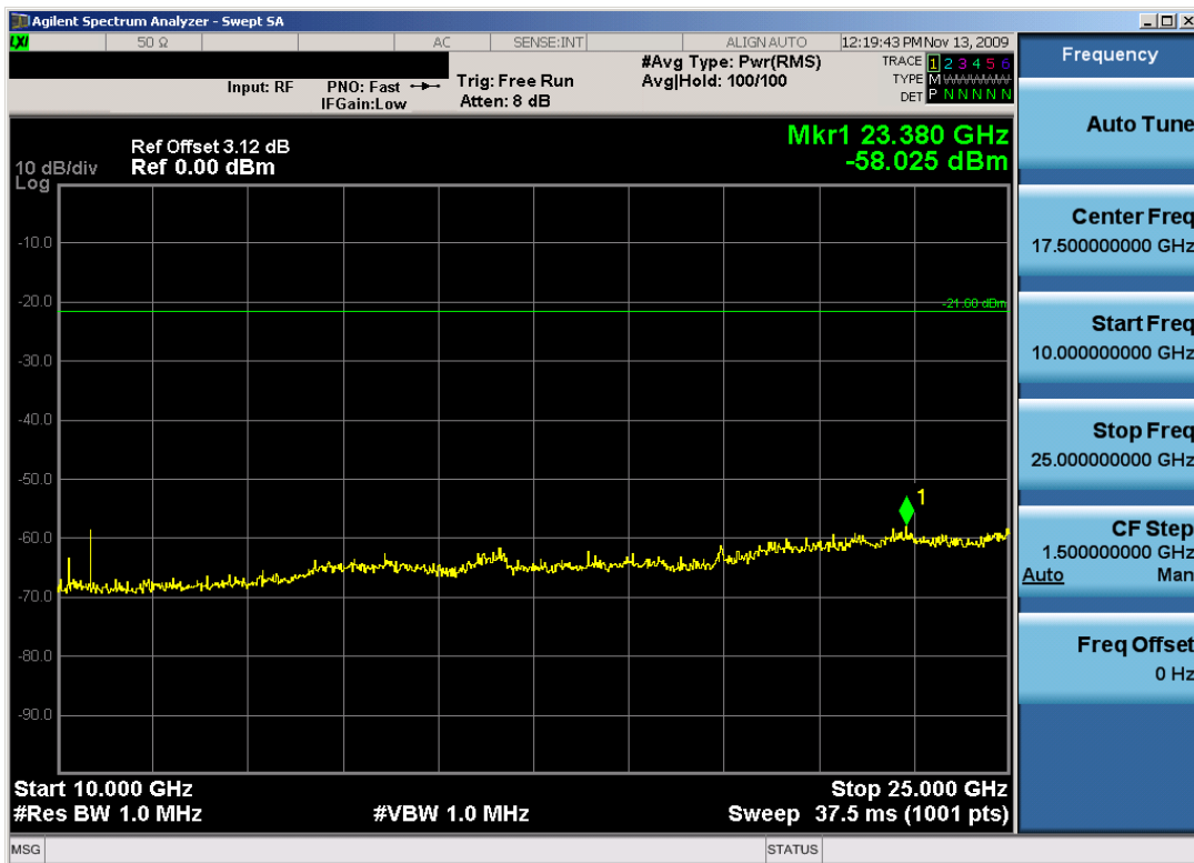
Plot 6-15. Conducted Spurious Plot (Bluetooth – Ch. 39)
