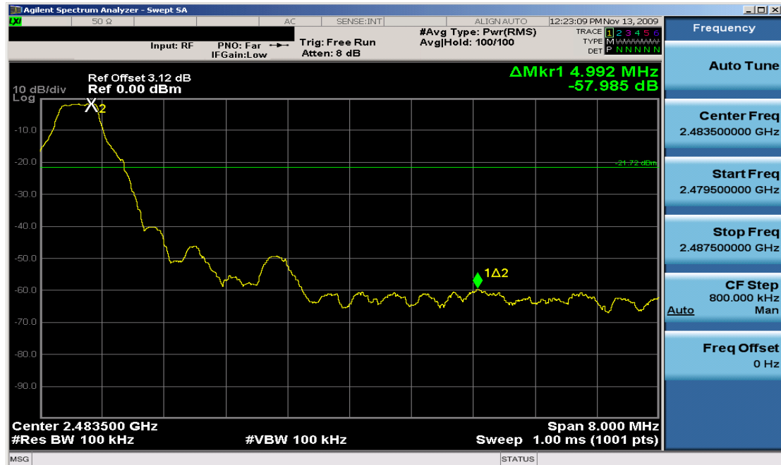
Plot 6-5. Band Edge Plot (Bluetooth – Ch. 78)
