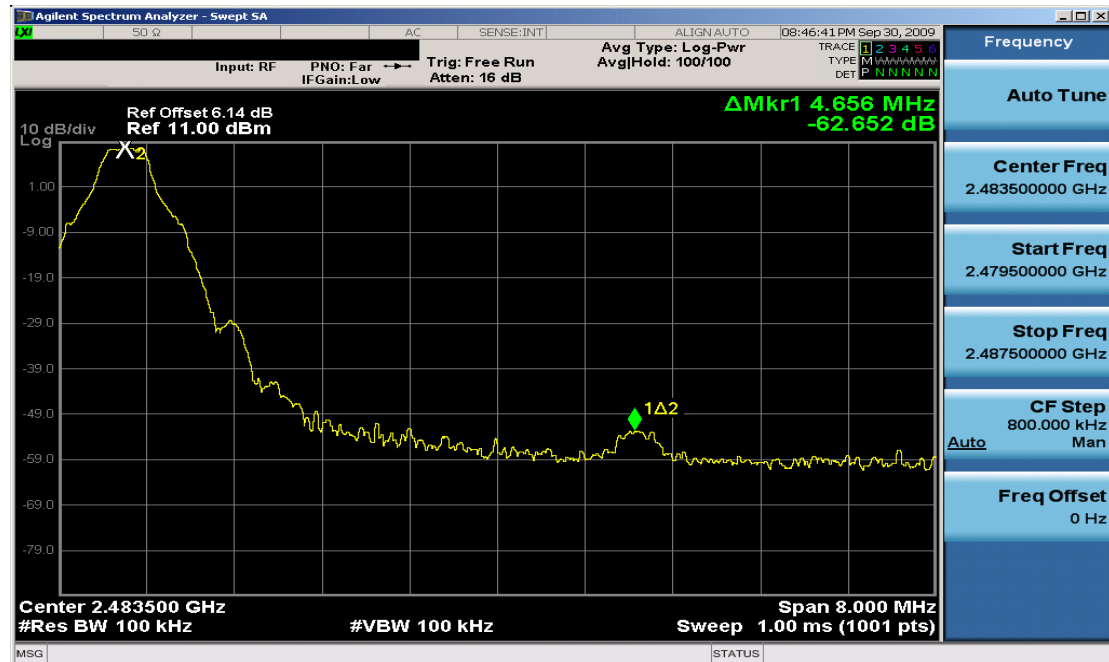
Plot 6-5. Band Edge Plot (Bluetooth – Ch. 78)
