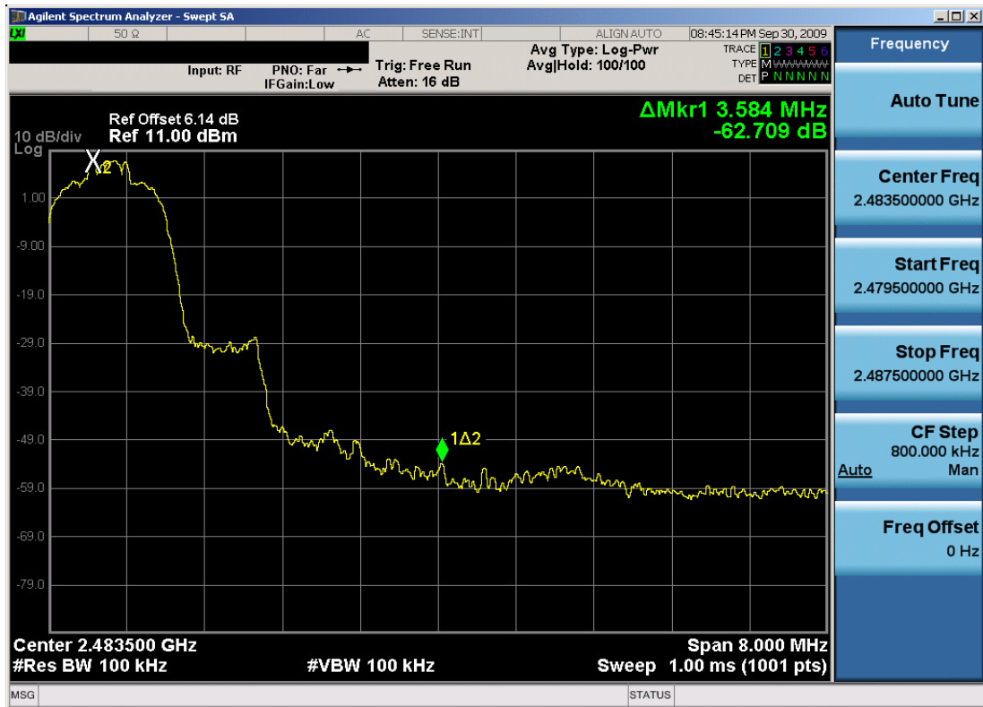
Plot 6-7. Band Edge Plot (Bluetooth 2.1 with Enhanced Data Rates – Ch. 78)
