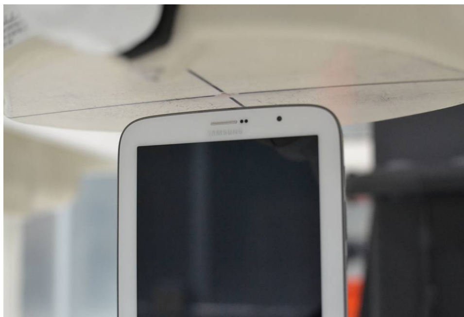
SAR Test Setup Photo 8 – Top Edge at 0.6 cm
