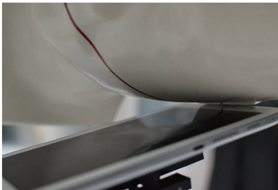
SAR Test Setup Photo 4 – Left Tilt
