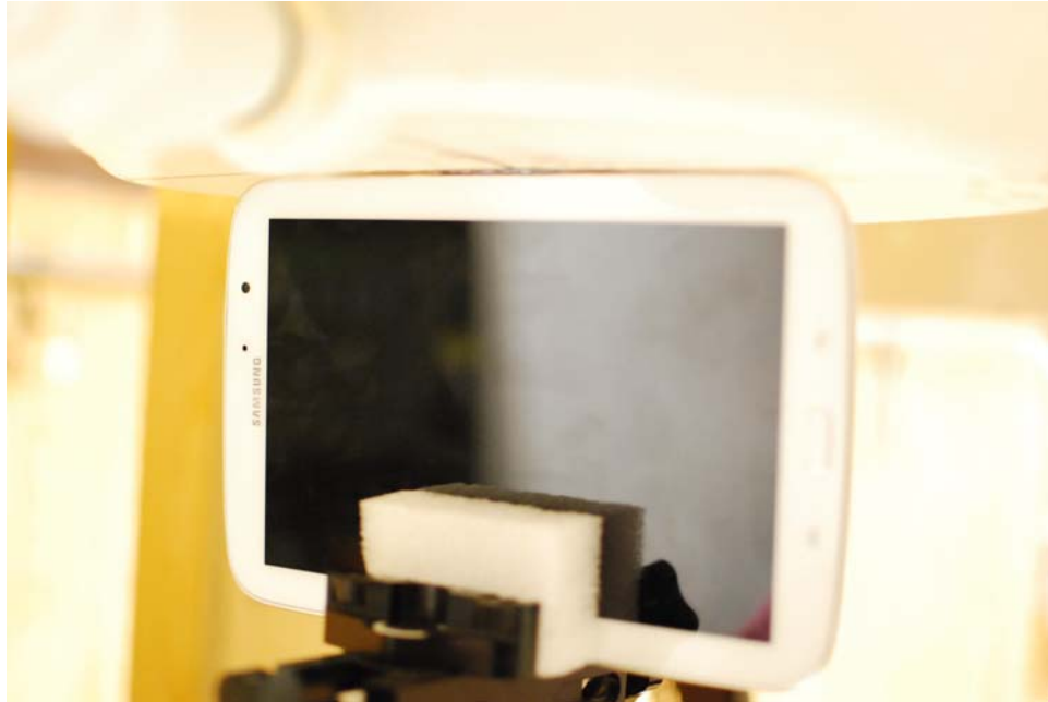
SAR Test Setup Photo 3 – Right Edge at 0.0 cm
