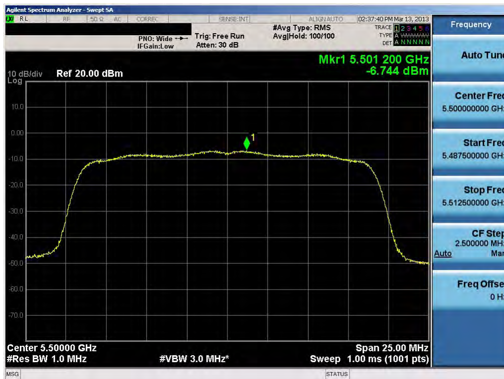
Plot 6-48. Peak Power Spectral Density Plot (20MHz BW 802.11n (UNII Band 3) – Ch. 100)
