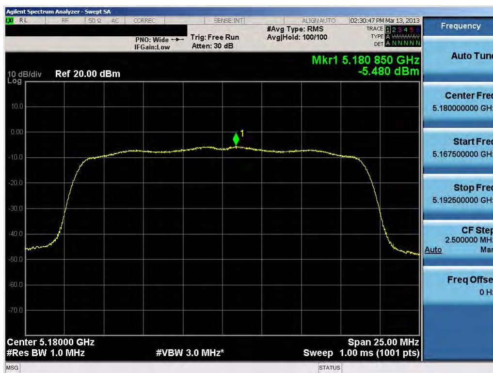
Plot 6-32. Peak Power Spectral Density Plot (20MHz BW 802.11n (UNII Band 1) – Ch. 36)
