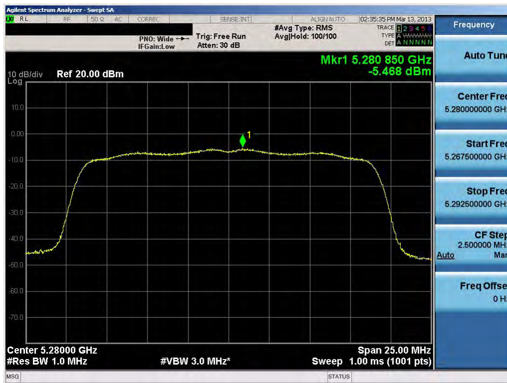
Plot 6-41. Peak Power Spectral Density Plot (20MHz BW 802.11n (UNII Band 2) – Ch. 56)
