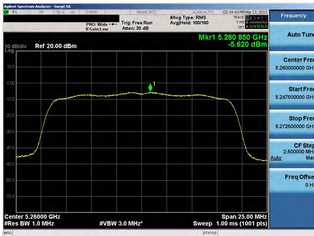
Plot 6-40. Peak Power Spectral Density Plot (20MHz BW 802.11n (UNII Band 2) – Ch. 52)
