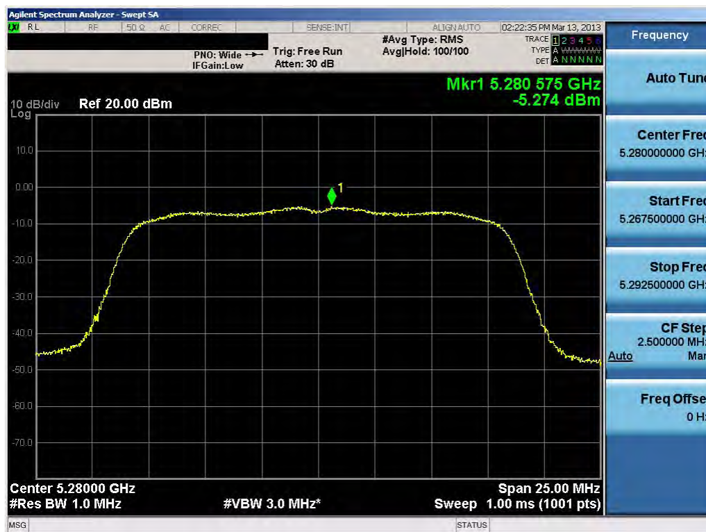
Plot 6-38. Peak Power Spectral Density Plot (802.11a (UNII Band 2) – Ch. 56)
