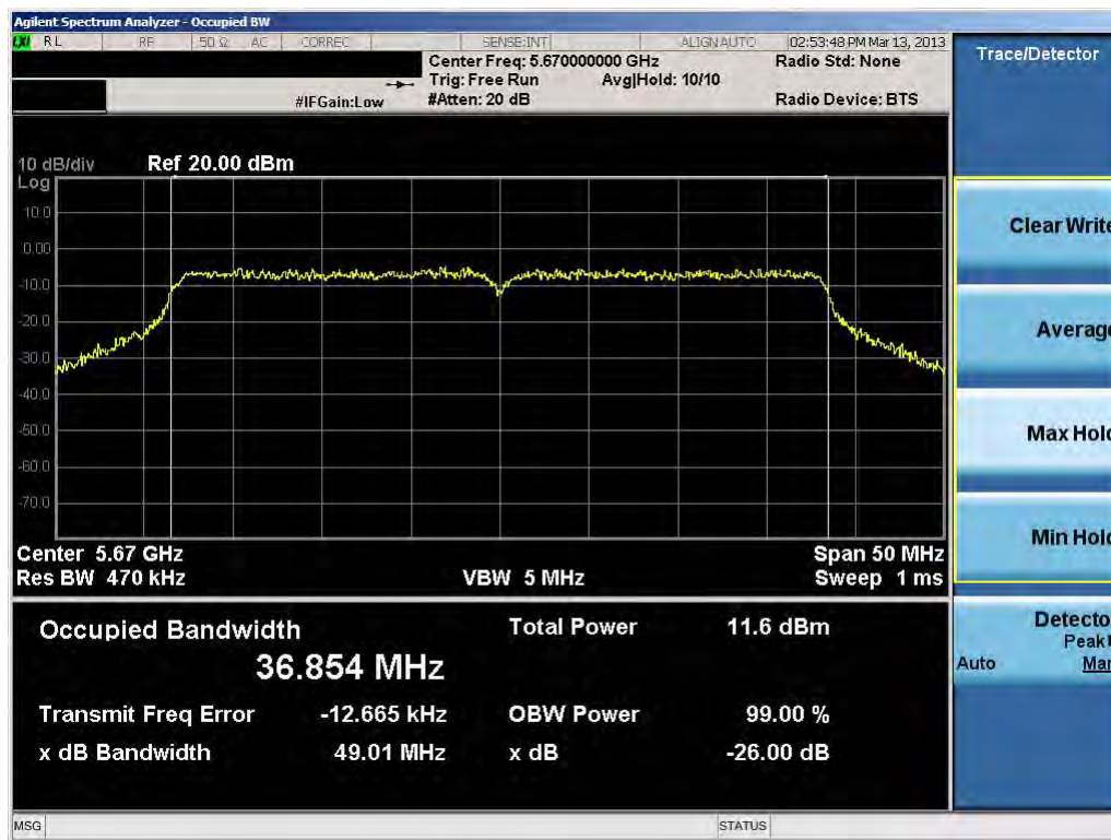
Plot 6-25. 26dB Bandwidth Plot (40MHz BW 802.11n (UNII Band 3) – Ch. 134)
