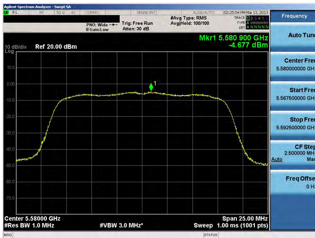
Plot 6-46. Peak Power Spectral Density Plot (802.11a (UNII Band 3) – Ch. 116)
