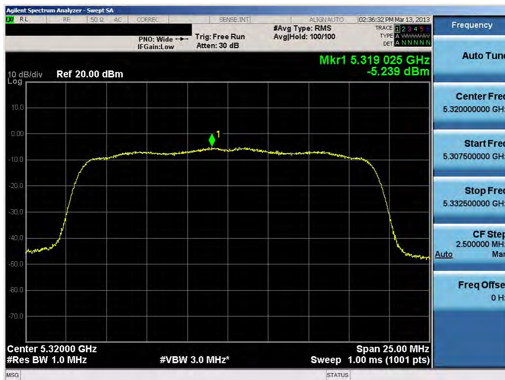
Plot 6-42. Peak Power Spectral Density Plot (20MHz BW 802.11n (UNII Band 2) – Ch. 64)
