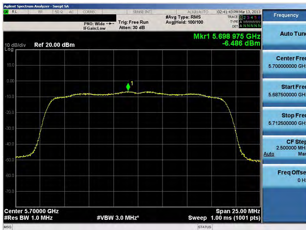
Plot 6-50. Peak Power Spectral Density Plot (20MHz BW 802.11n (UNII Band 3) – Ch. 140)
