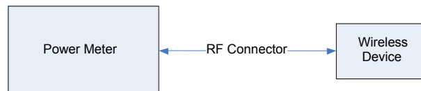
Figure 12-2 Power Measurement Setup
