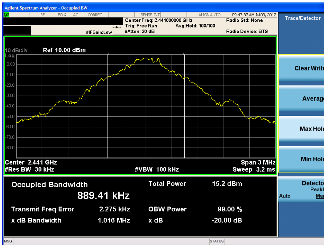
Plot 6-2. 20dB Bandwidth Plot (Bluetooth, 1Mbps – Ch. 39)
