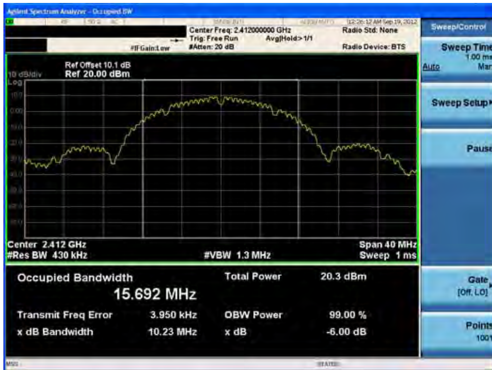
6dB Bandwidth plot (802.11b-CH 6)
