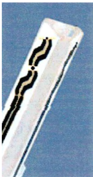
Figure 3.3 ET3DV6 E-field Probe
