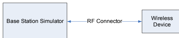
Figure 8-2 Power Measurement Setup
