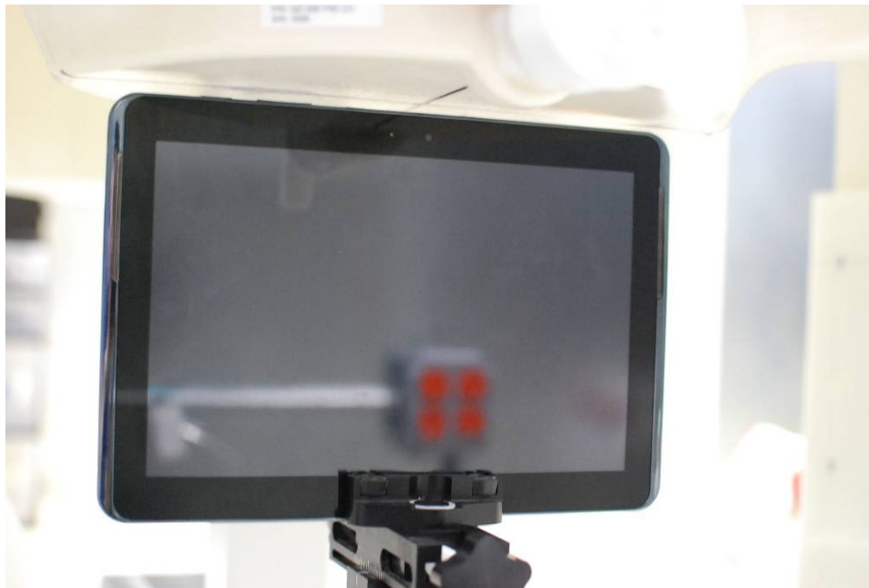
SAR Test Setup Photo 4 – Top Edge at 0.5 cm
