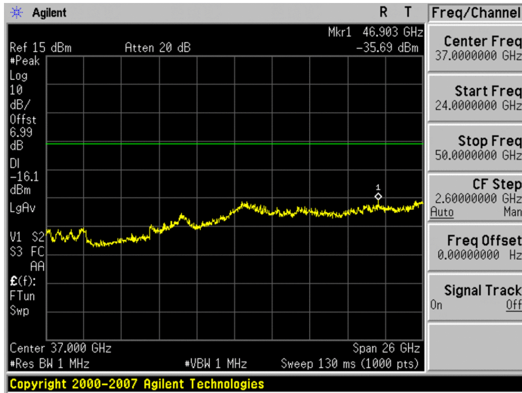
Plot 6-52. Conducted Spurious Plot (802.11a – Ch. 165)
