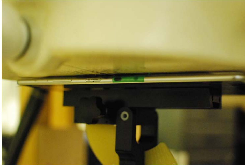
SAR Test Setup Photo 1: Back at 0.0 cm
