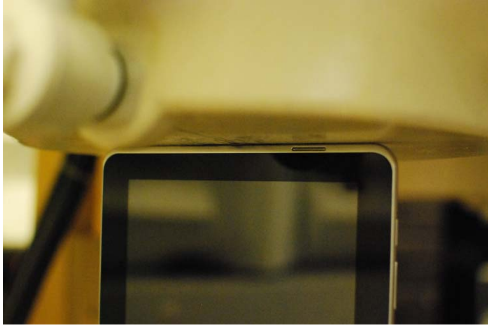
SAR Test Setup Photo 3: Left at 0.0 cm
