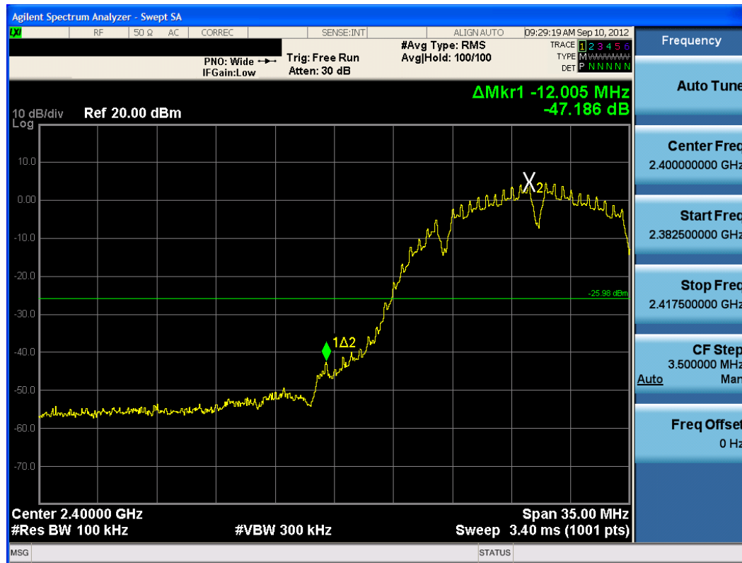
Plot 6-35. Band Edge Plot (802.11b – Ch. 1)
