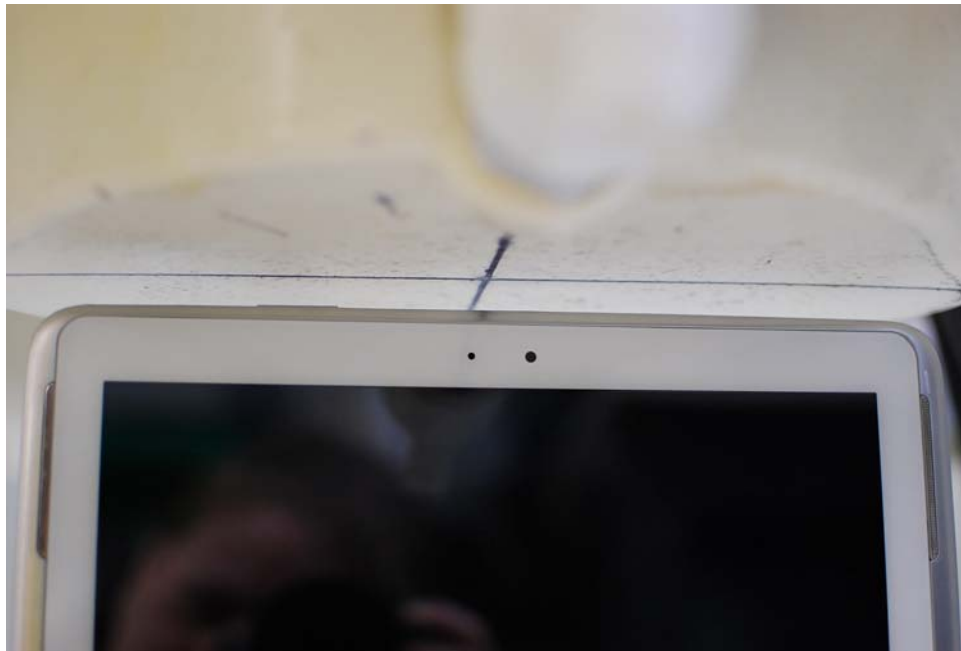
SAR Test Setup Photo 4: Top at 1.0 cm
