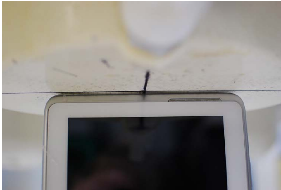
SAR Test Setup Photo 6: Left at 0.0 cm
