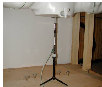
Figure 10-2 System Verification Setup Photo
