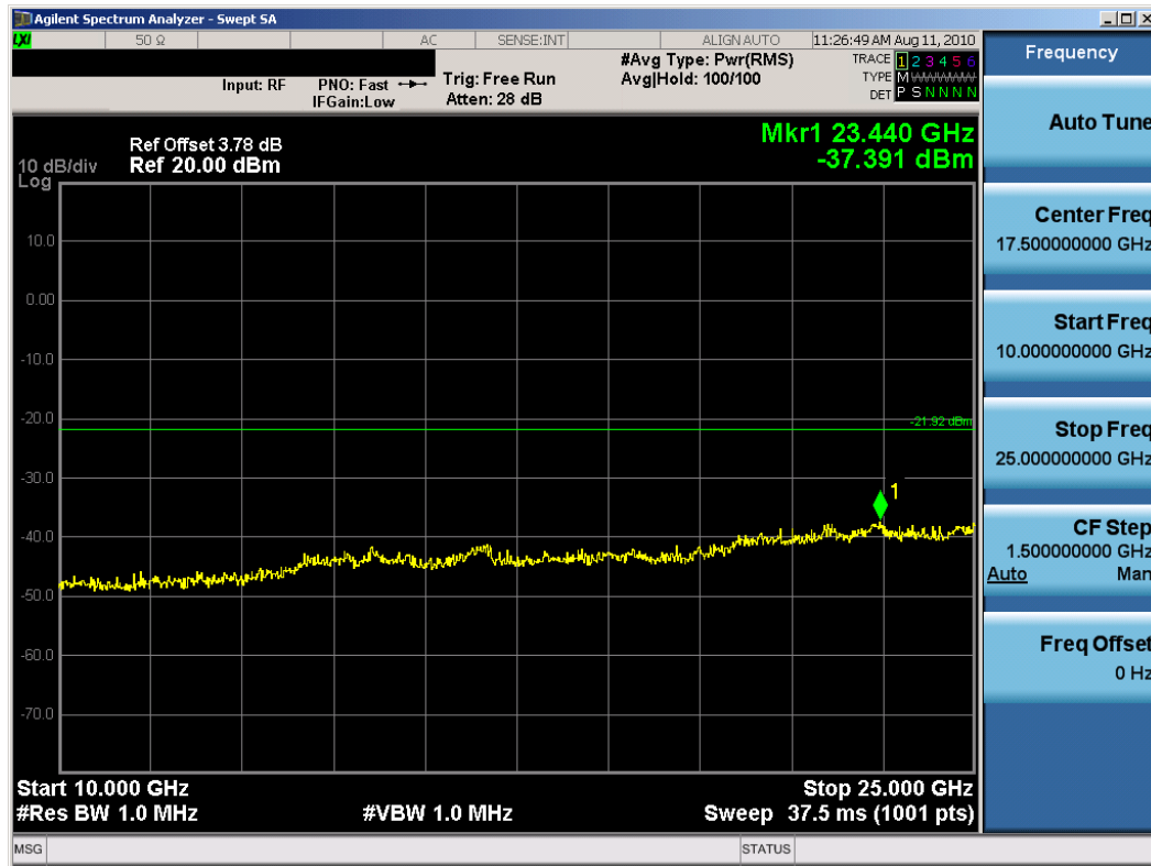
Plot 6-46. Conducted Spurious Plot (802.11b – Ch. 11)
