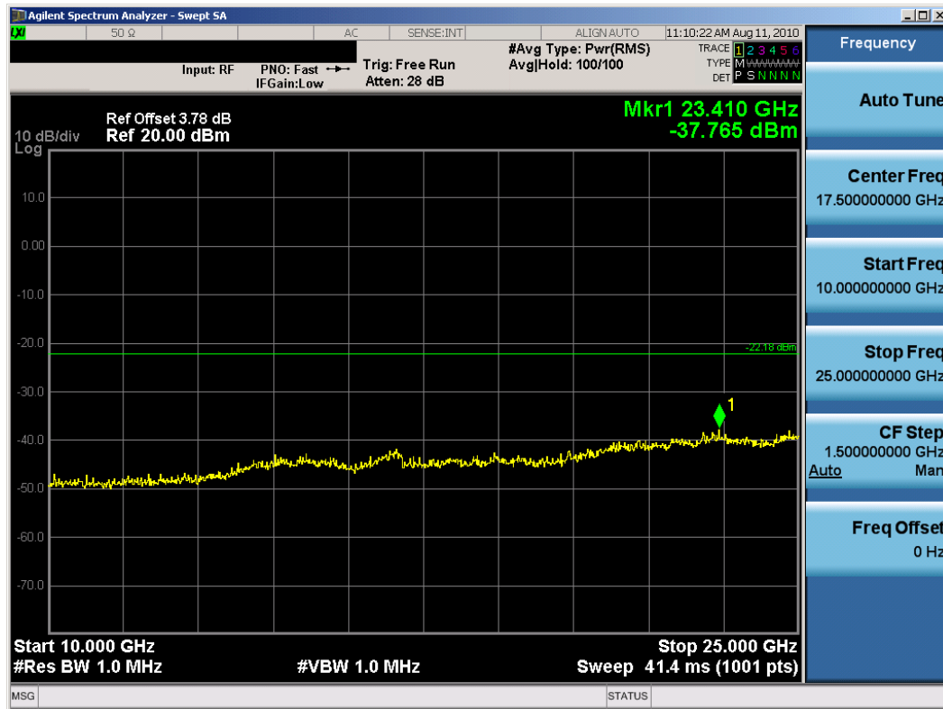
Plot 6-42. Conducted Spurious Plot (802.11b - Ch. 1)
