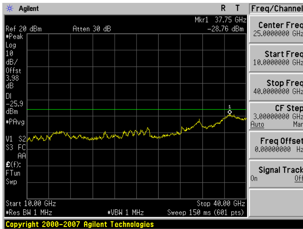
Plot 6-52. Conducted Spurious Plot (802.11a – Ch. 161)
