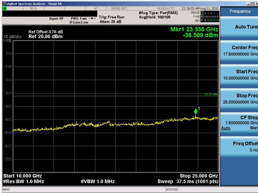
Plot 6-44. Conducted Spurious Plot (802.11b – Ch. 6)
