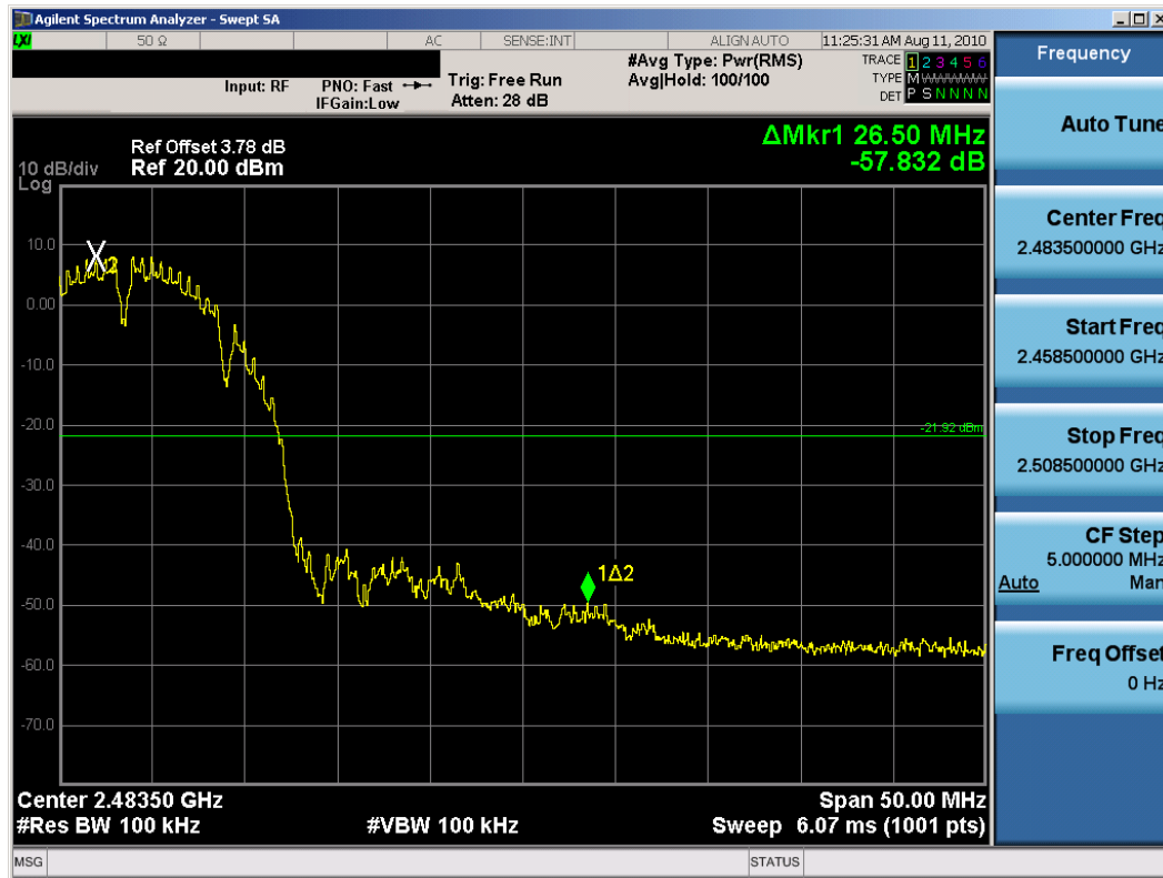
Plot 6-32. Band Edge Plot (802.11b – Ch. 11)
