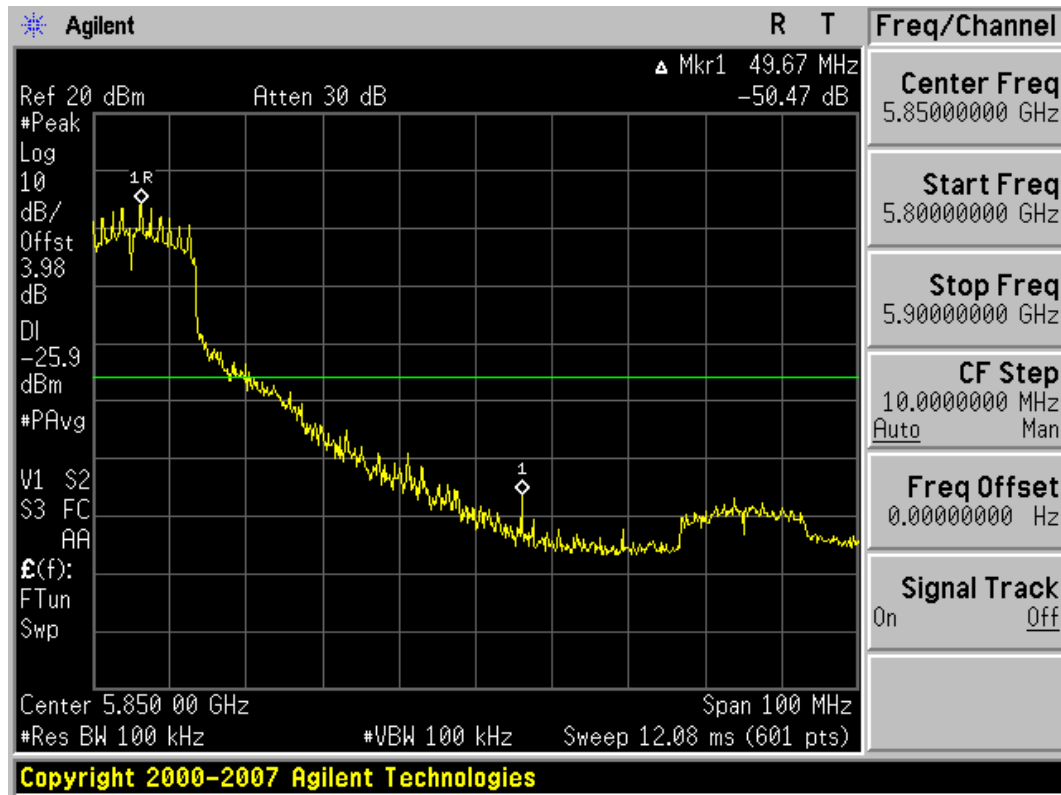
Plot 6-36. Band Edge Plot (802.11a – Ch. 161)
