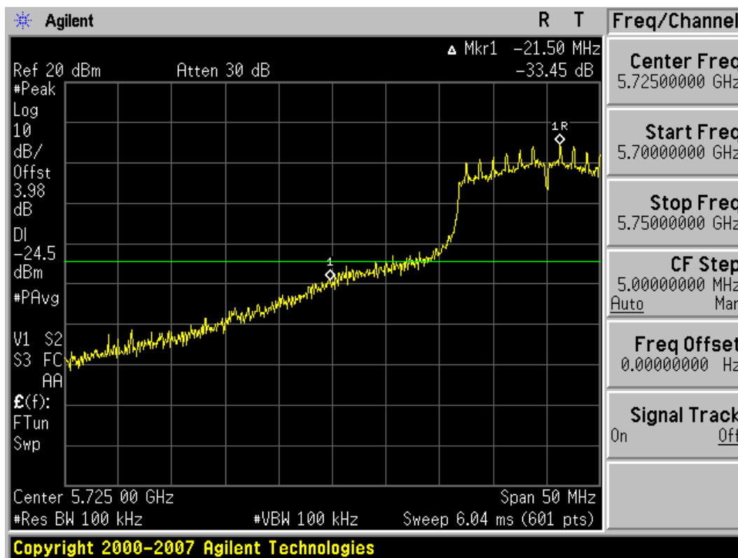
Plot 6-35. Band Edge Plot (802.11a – Ch. 149)
