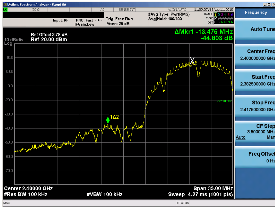
Plot 6-31. Band Edge Plot (802.11b – Ch. 1)
