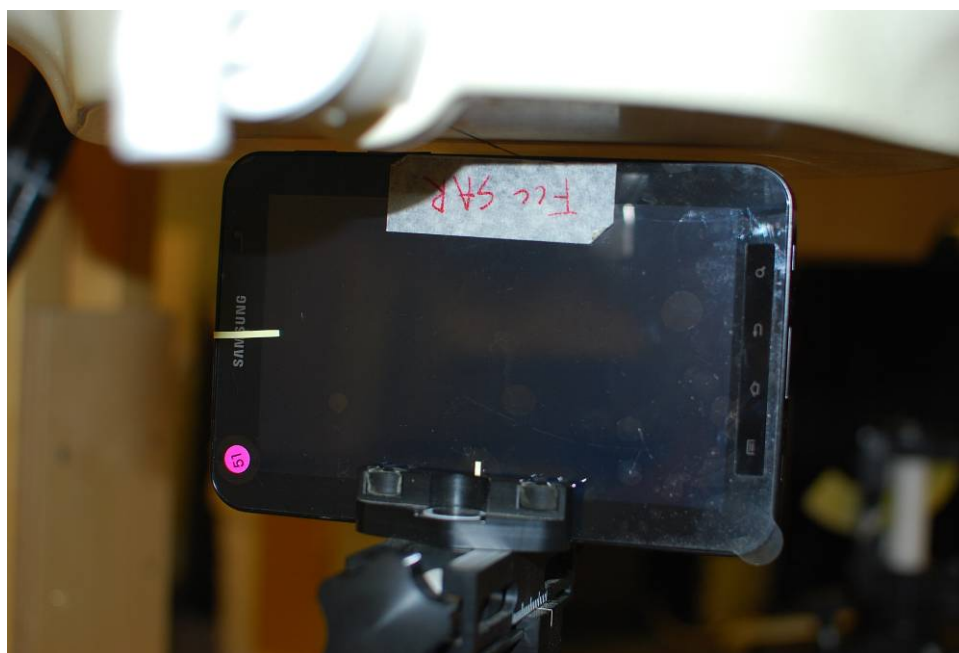
Figure 20-6 SAR Test Setup Photo 5 – Right at 0.5 cm
