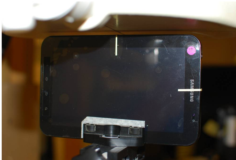
Figure 20-5 SAR Test Setup Photo 4 – Left at 0.5 cm
