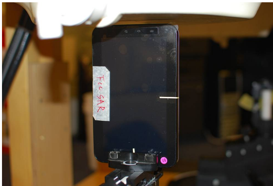
Figure 20-7 SAR Test Setup Photo 6 – Bottom at 0.5 cm
