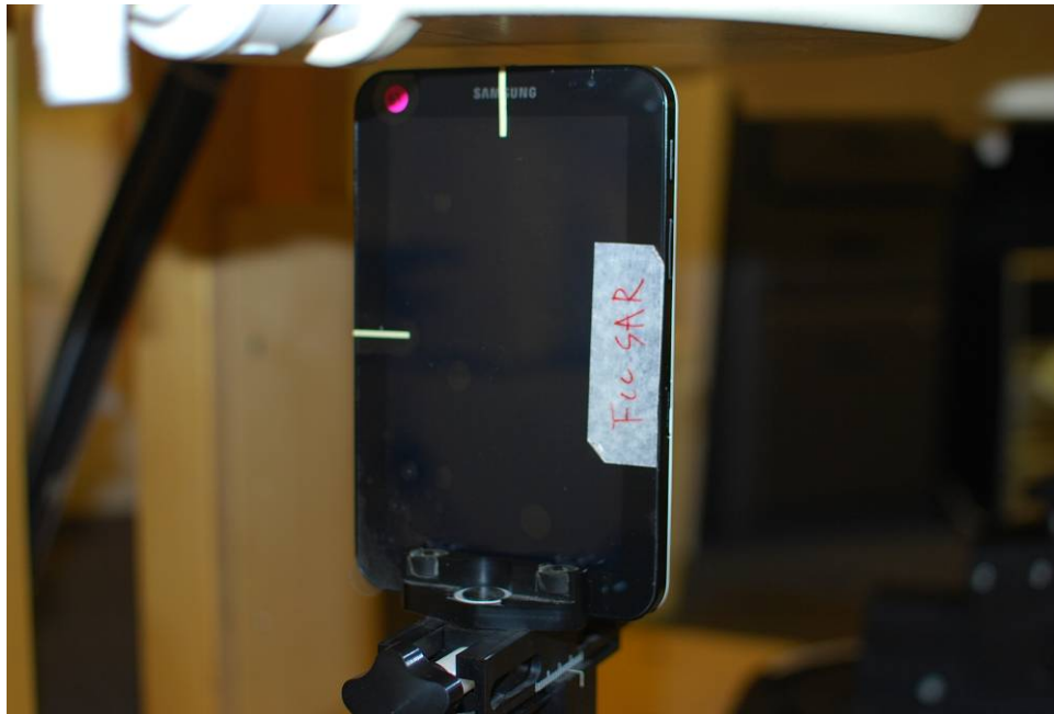
Figure 20-3 SAR Test Setup Photo 3 – Top at 0.75 cm
