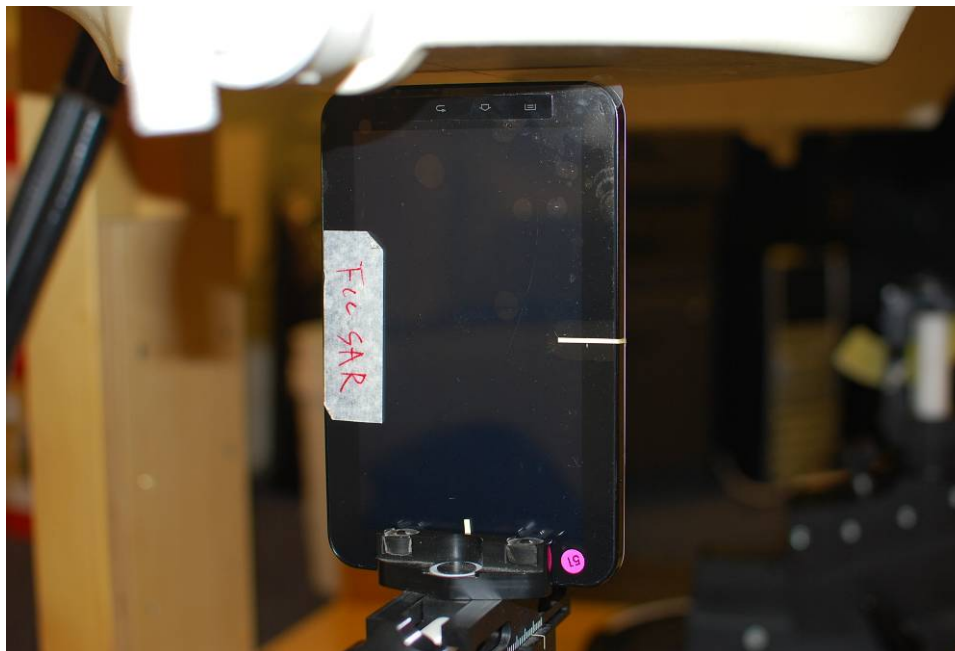
Figure 20-7 SAR Test Setup Photo 6 – Bottom at 0.5 cm
