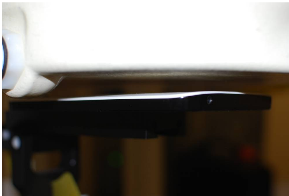
Figure 20-2 SAR Test Setup Photo 2 – Back Side at 1.0 cm (with power back-off inactive)
