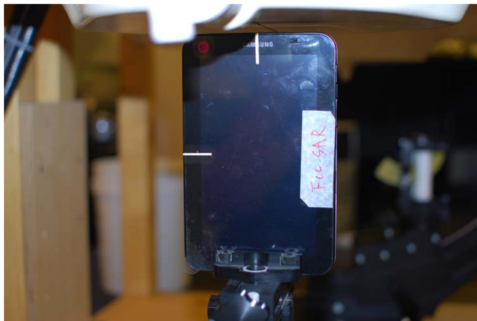
Figure 20-4 SAR Test Setup Photo 3 – Top at 0.5 cm
