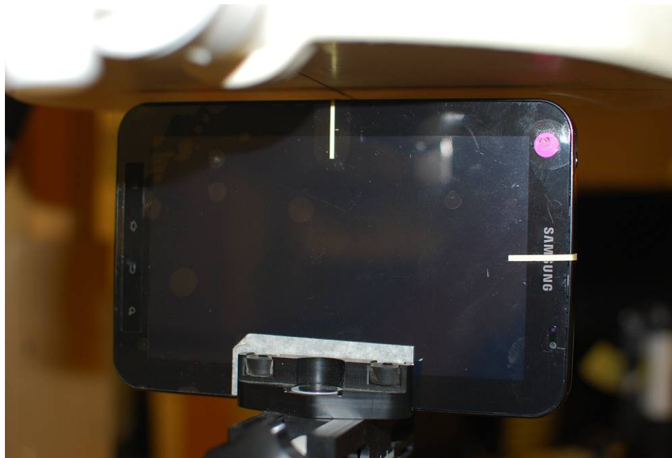
Figure 20-5 SAR Test Setup Photo 4 – Left at 0.5 cm
