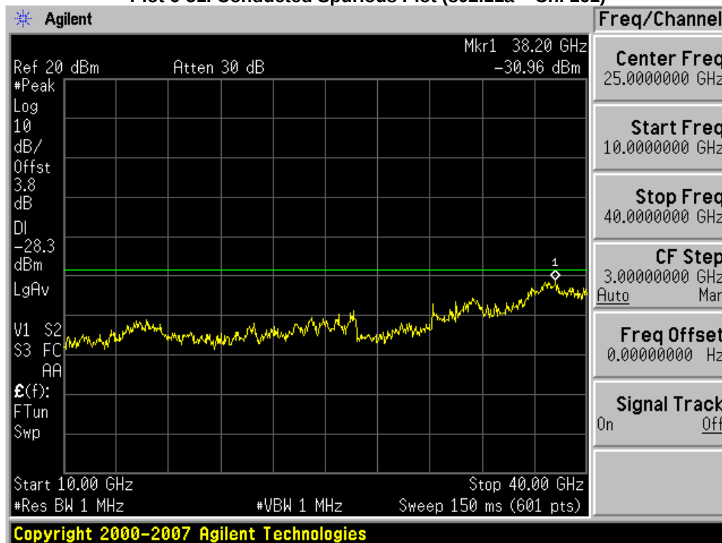
Plot 6-52. Conducted Spurious Plot (802.11a - Ch. 161)
