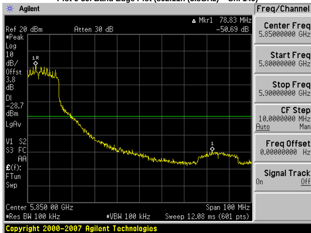
Plot 6-40. Band Edge Plot (802.11n (5.8GHz) – Ch. 161)
