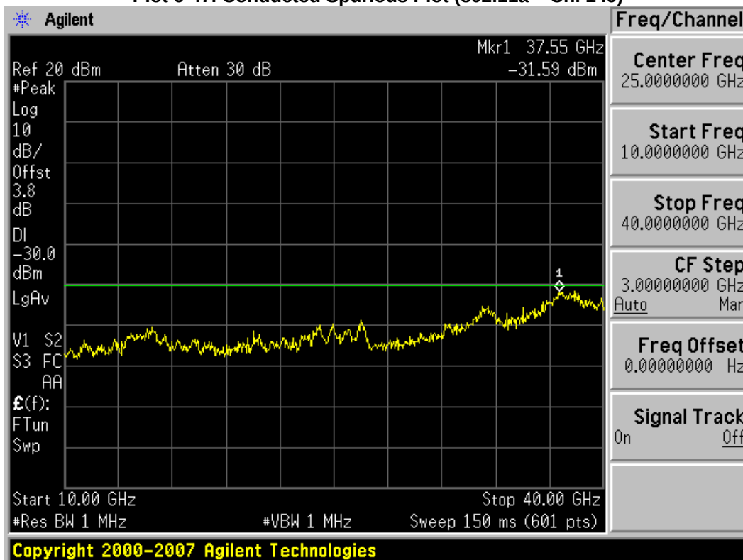
Plot 6-48. Conducted Spurious Plot (802.11a - Ch. 149)
