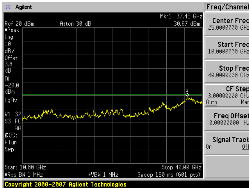
Plot 6-50. Conducted Spurious Plot (802.11a – Ch. 157)
