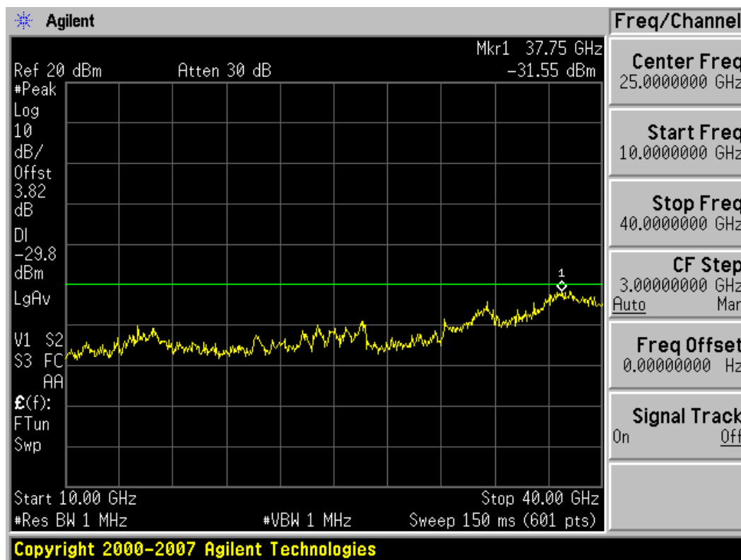
Plot 6-48. Conducted Spurious Plot (802.11a – Ch. 149)
