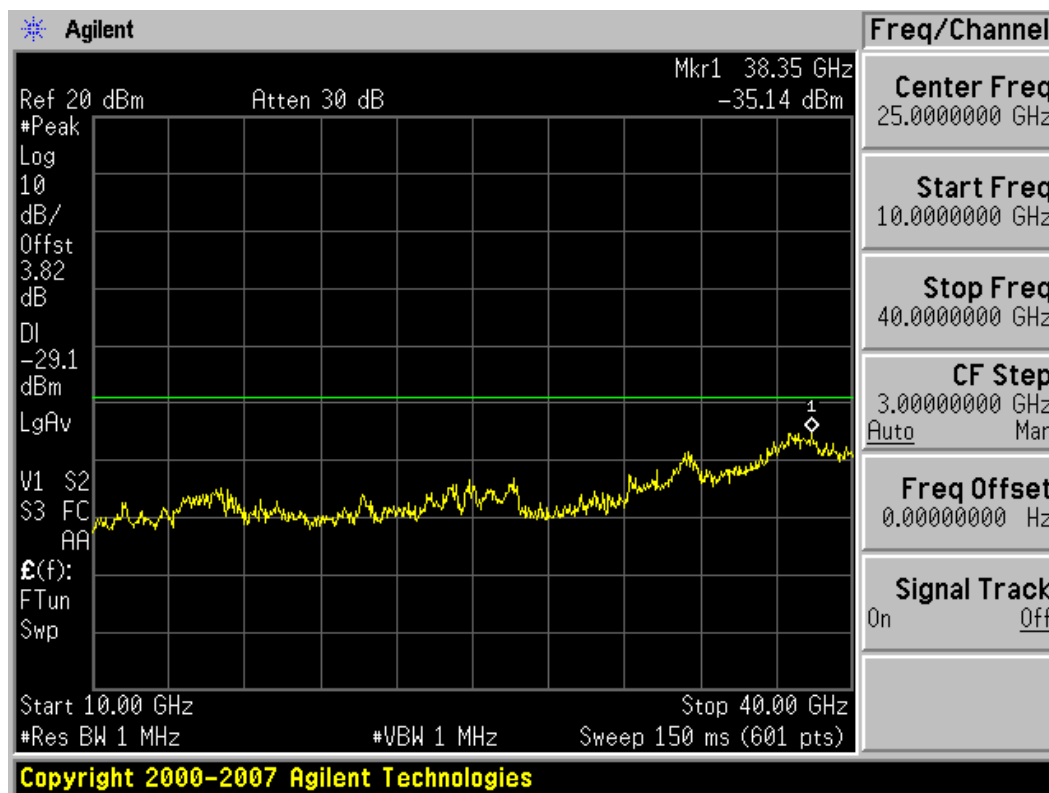
Plot 6-50. Conducted Spurious Plot (802.11a – Ch. 157)
