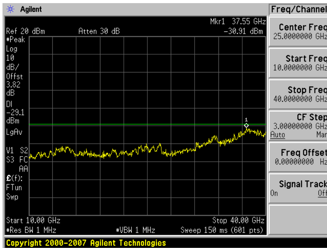
Plot 6-52. Conducted Spurious Plot (802.11a – Ch. 161)
