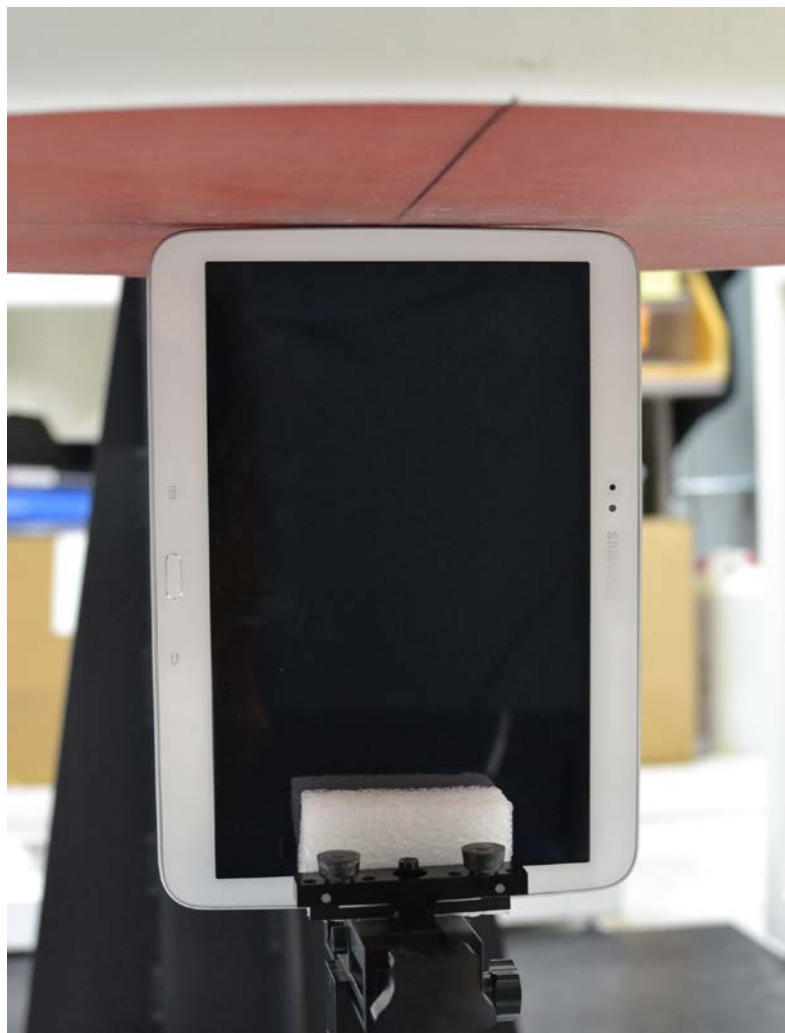
SAR Test Setup Photo 3 - Left Side at 0.0 cm
