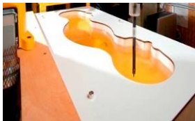
Figure 6-2 SAM Phantom with Simulating Tissue
