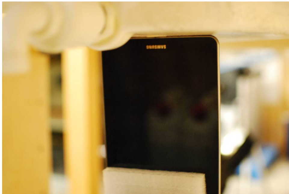
SAR Test Setup Photo 8 – Bottom at 0.0 cm
