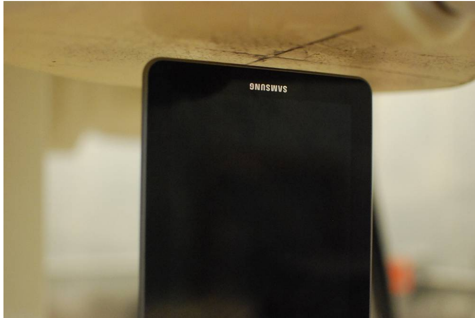
SAR Test Setup Photo 8 – Bottom at 0.5 cm
