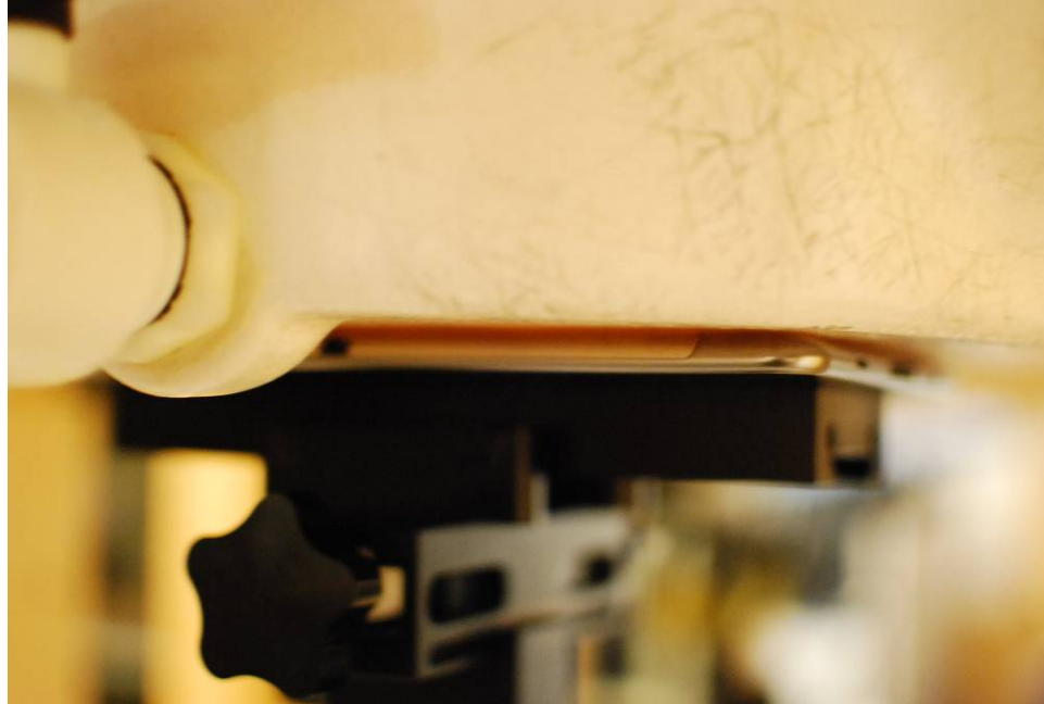
SAR Test Setup Photo 5 - Back at 0.0 cm
