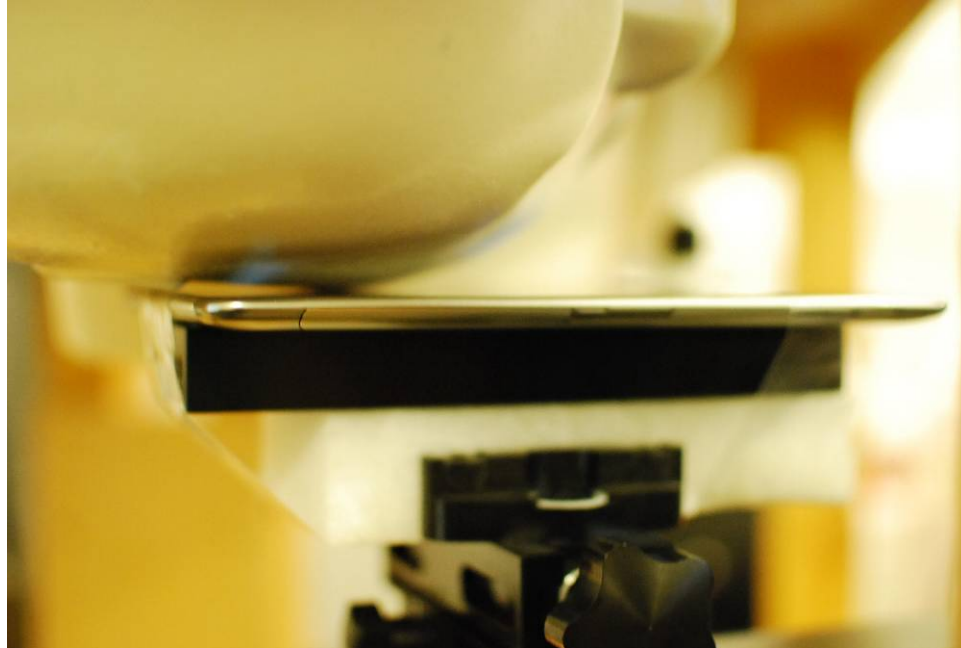
SAR Test Setup Photo 1 – Right Touch
