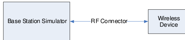
Figure 11-1 Power Measurement Setup
