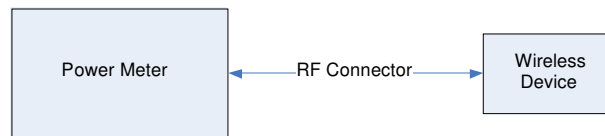
Figure 12-1 Power Measurement Setup
