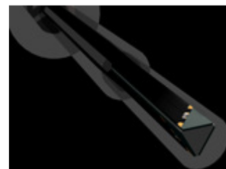
Figure 4-3 Triangular Probe Configuration
