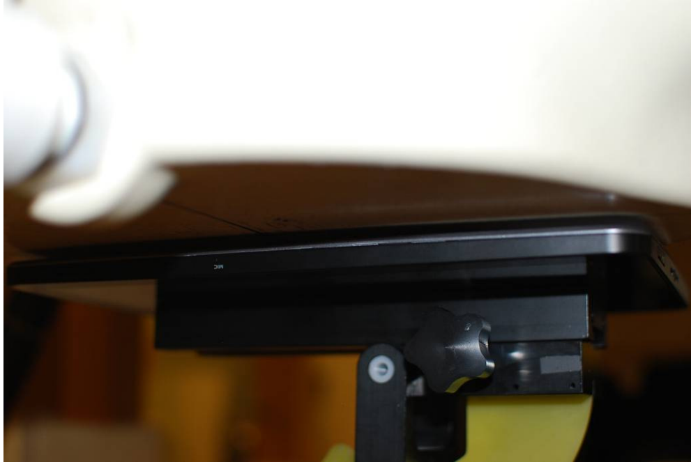
Figure 20-1 SAR Test Setup Photo – Back at 0.0 cm
