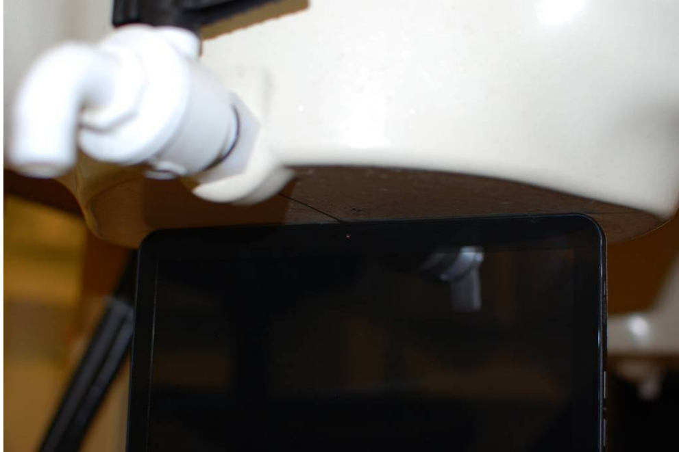
Figure 20-3 SAR Test Setup Photo – Top at 0.0 cm
