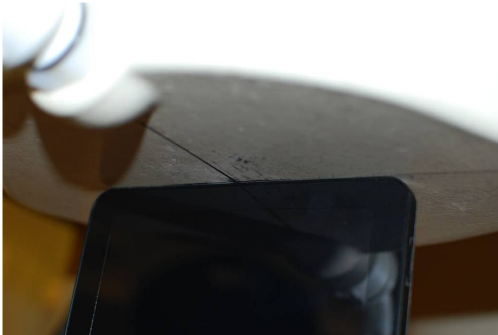
Figure 20-7 SAR Test Setup Photo – Left at 0.0 cm
