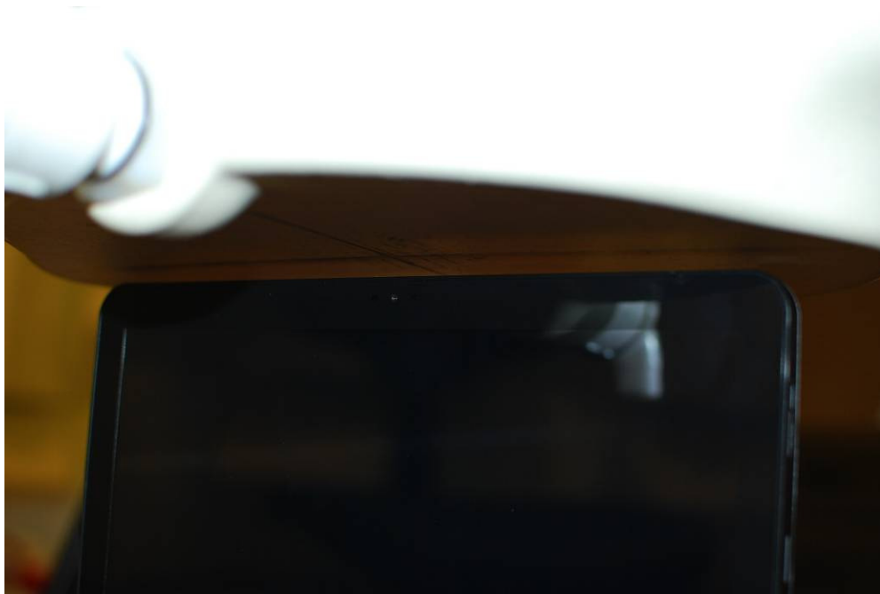
Figure 20-4 SAR Test Setup Photo – Top at 0.5 cm
