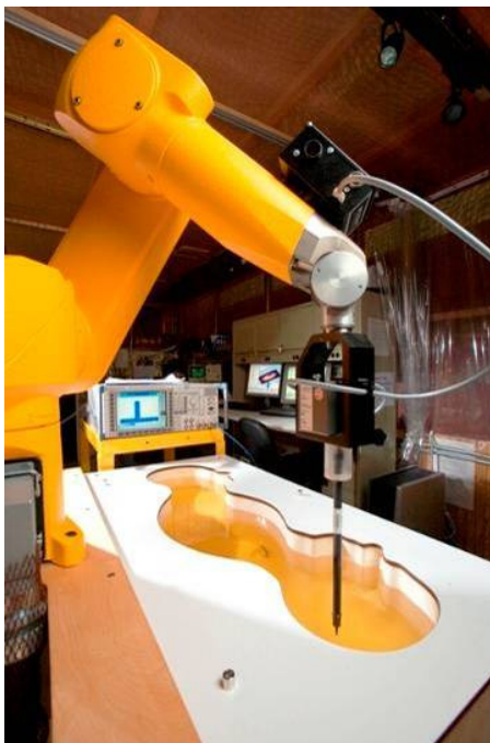
Figure 3-2 SAR Measurement System
