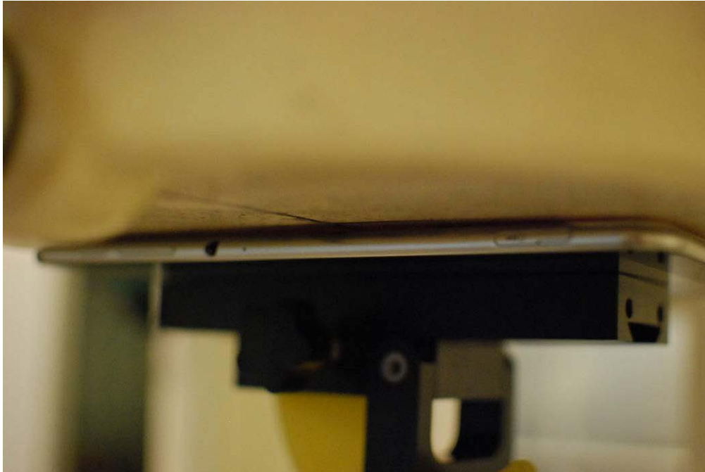
SAR Test Setup Photograph 1 – Back at 0.0 cm
