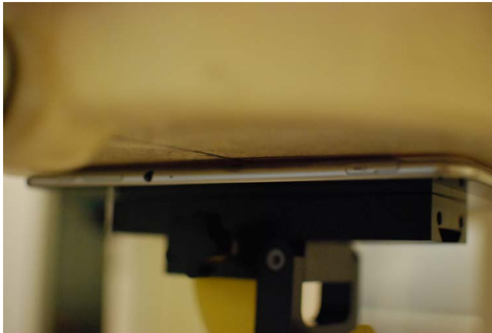
SAR Test Setup Photo 2: Back at 0.0 cm
