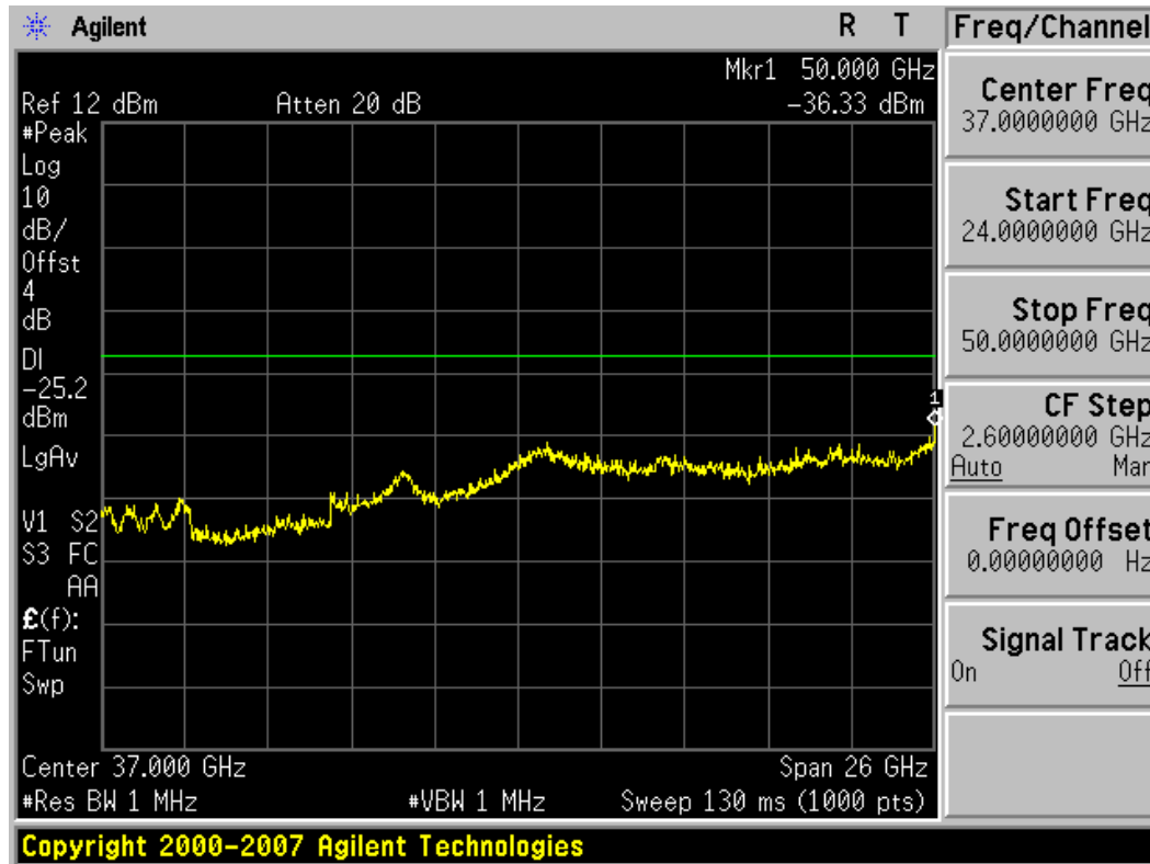
Plot 6-50. Conducted Spurious Plot (802.11a – Ch. 157)
