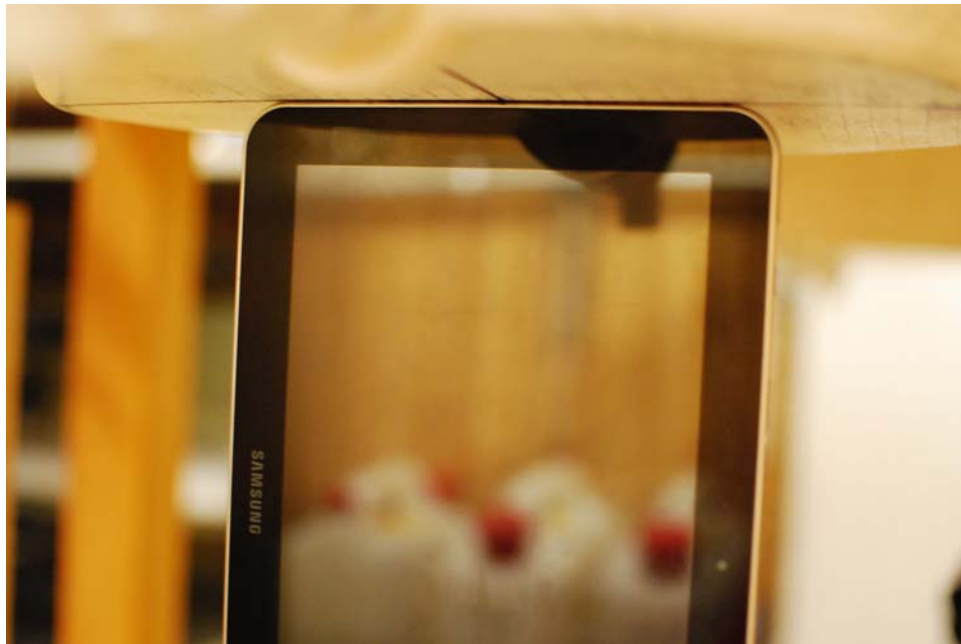
SAR Test Setup Photo 6: Left at 0.0 cm
