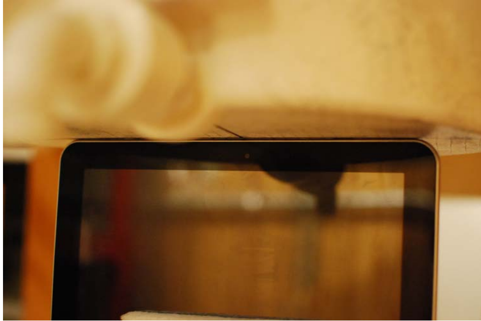
SAR Test Setup Photo 3: Top at 0.0 cm
