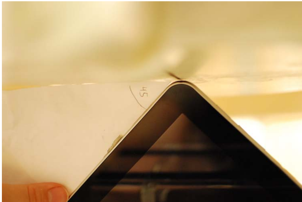
SAR Test Setup Photo 8: 45° Vertex at 0.0 cm
