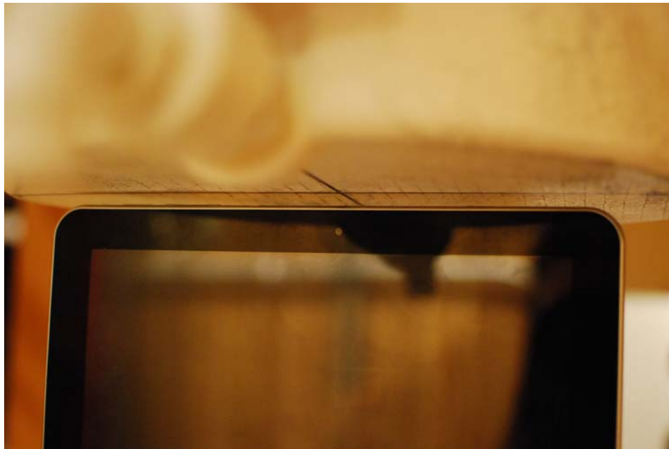
SAR Test Setup Photo 4: Top at 0.5 cm
