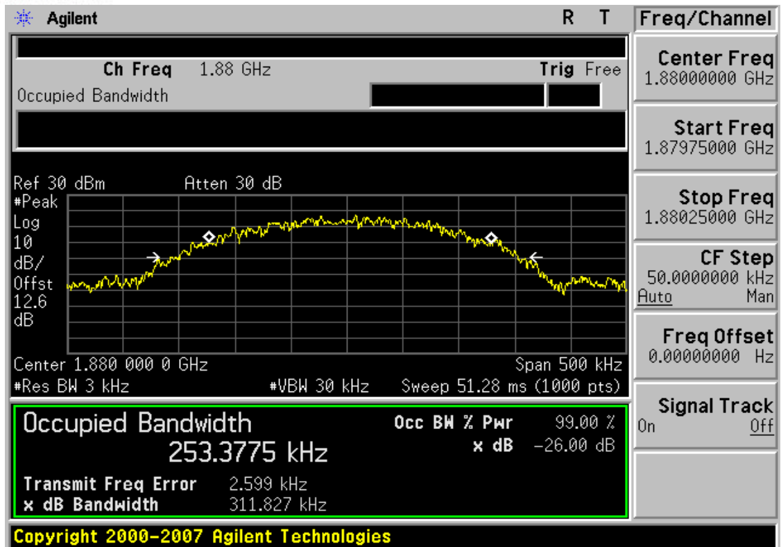
Plot 7-21. Occupied Bandwidth Plot (EDGE1900 Mode – Ch. 661)
