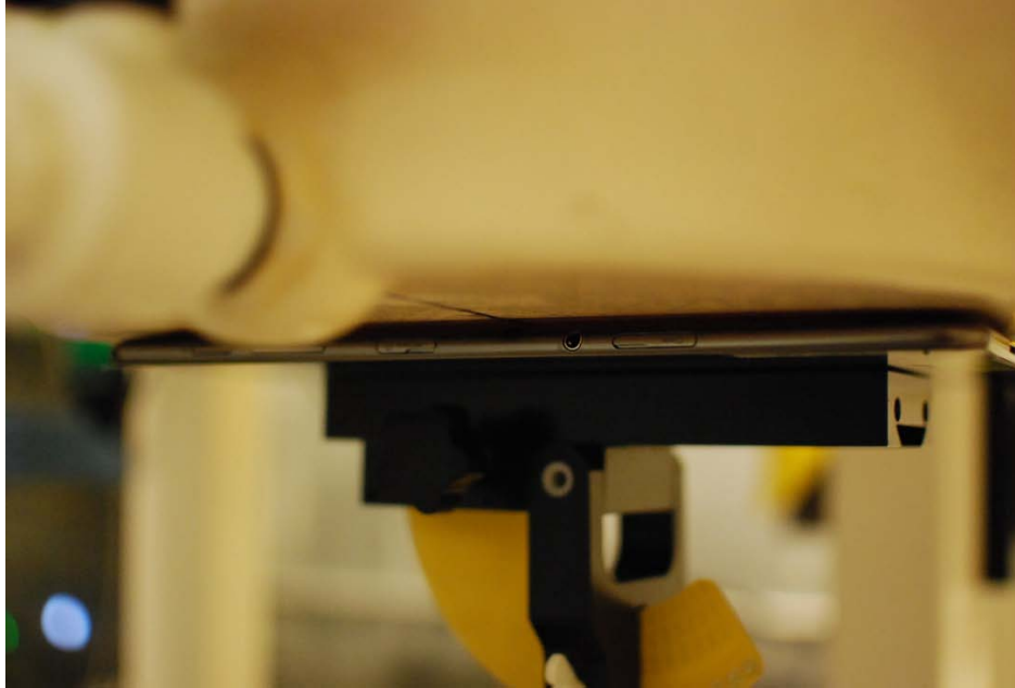
Figure 20-1 SAR Test Setup Photo 1 – Back at 0 cm
