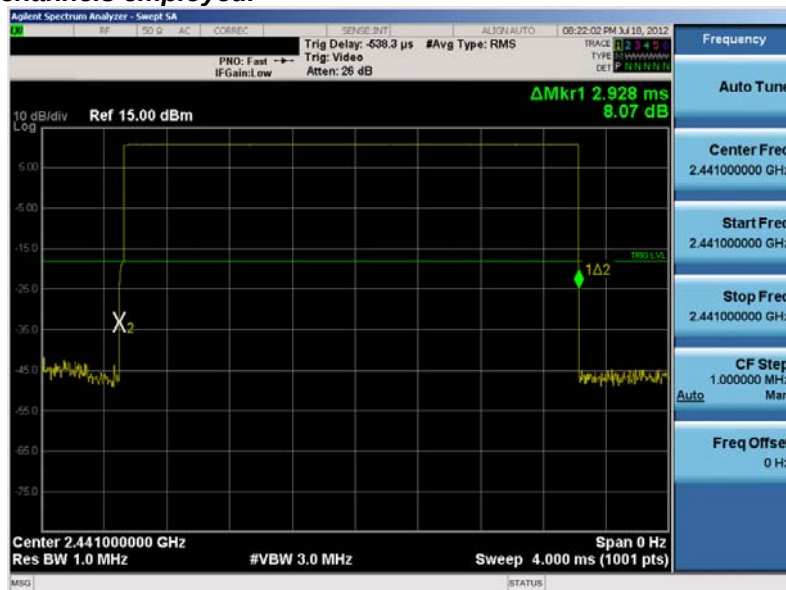
Plot 6-15. Time of Occupancy Plot (Bluetooth)
