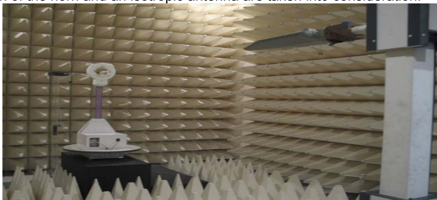
Figure2. Photograph of 3m Fully-Anechoic Chamber
