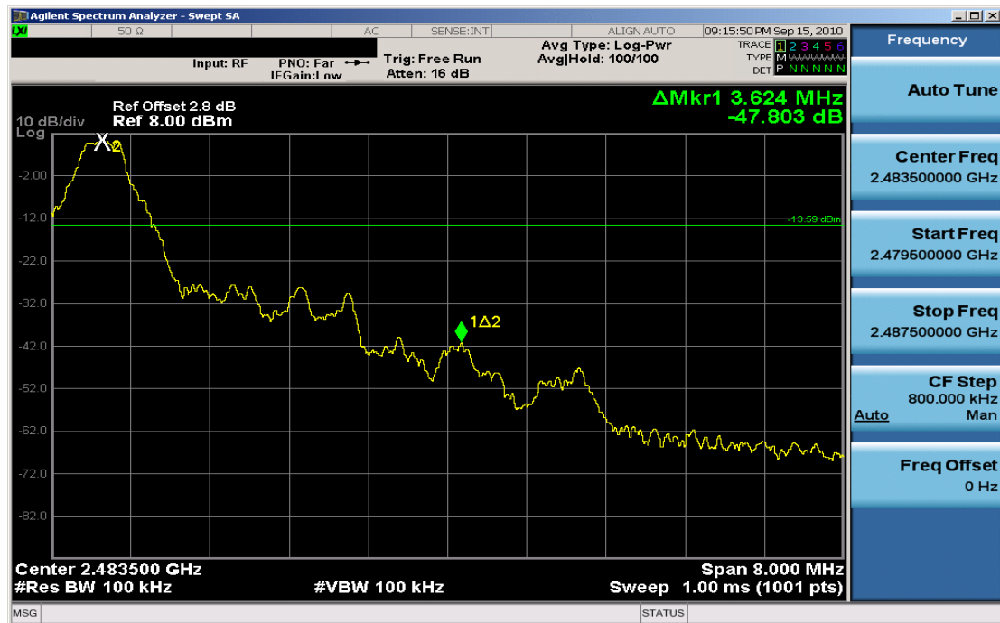
Plot 6-5. Band Edge Plot (Bluetooth – Ch. 78)
