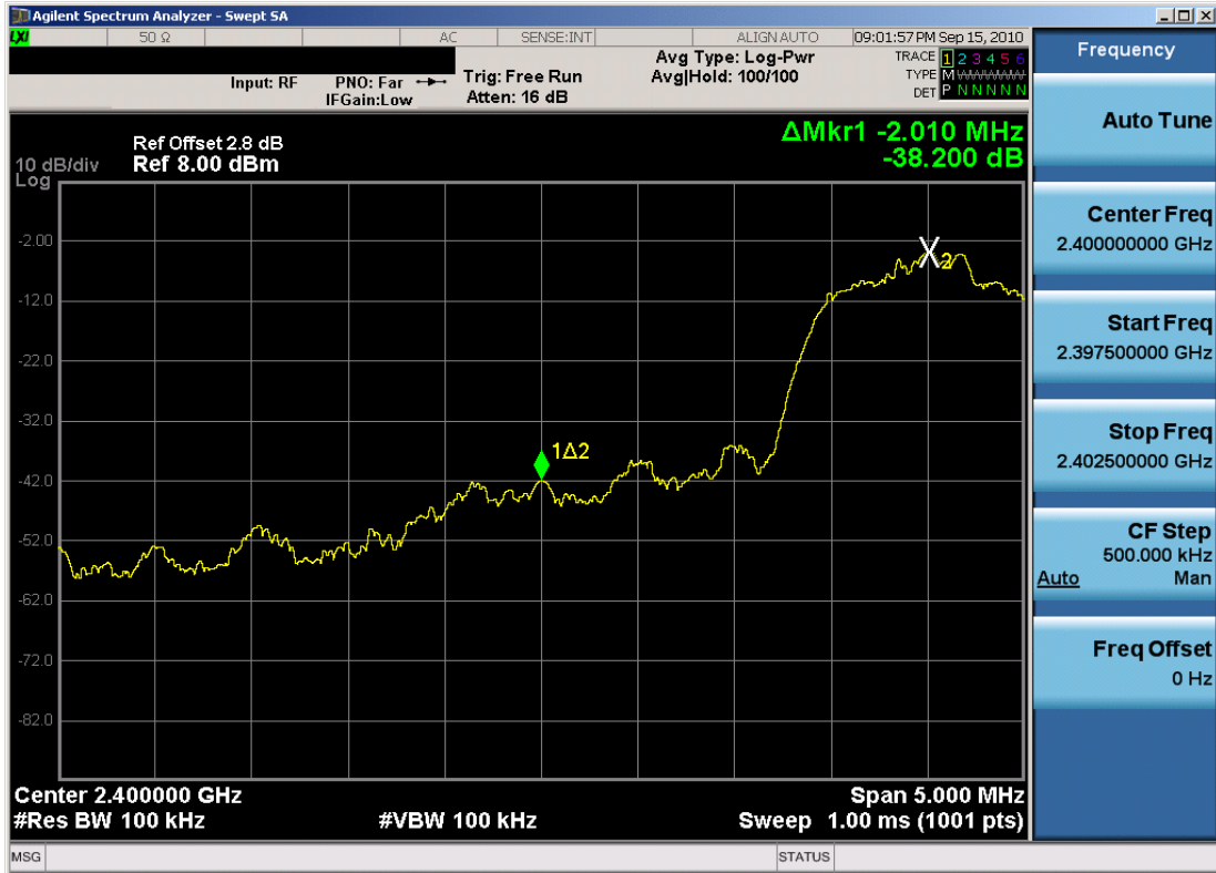
Plot 6-6. Band Edge Plot (Bluetooth (EDR) - Ch. 0)
