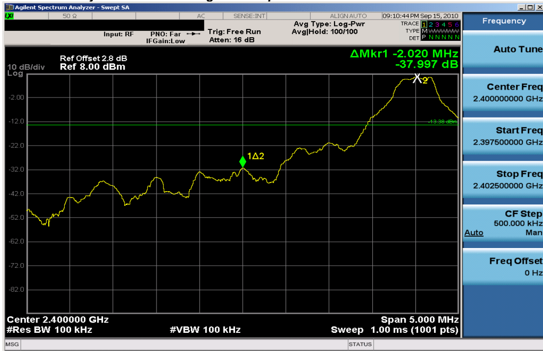
Plot 6-4. Band Edge Plot (Bluetooth – Ch. 0)
