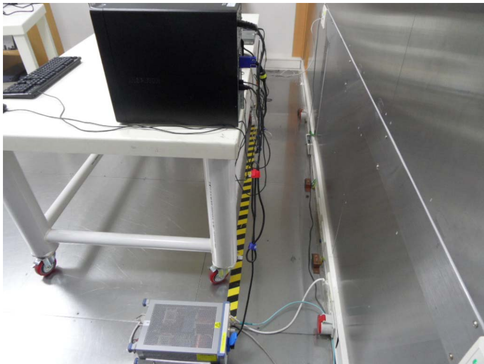
[ Conducted Disturbance – Rear ]
