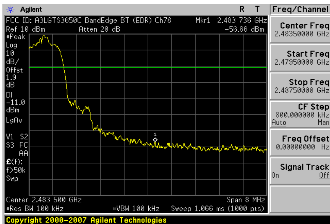
Plot 6-7. Band Edge Plot (Bluetooth 2.0 with Enhanced Data Rates – Ch. 78)
