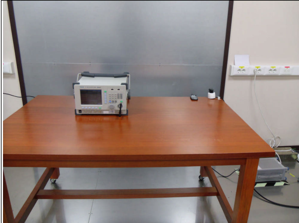
Photos of AC Power line conducted emission test.
