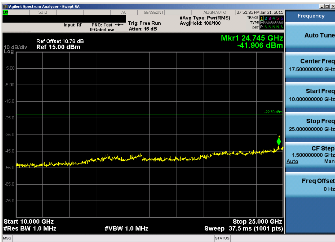
Plot 6-30. Conducted Spurious Plot (802.11b – Ch. 11)
