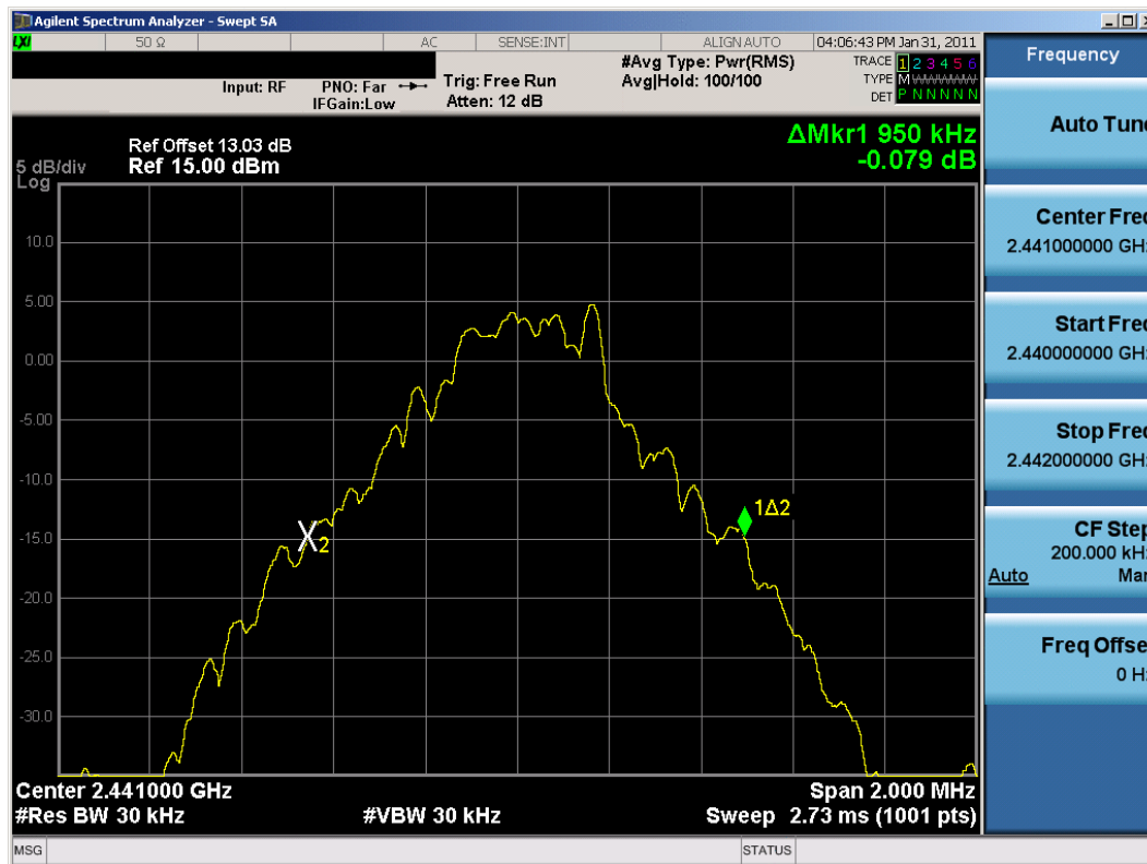
Plot 6-2. 20dB Bandwidth Plot (Bluetooth, 1Mbps – Ch. 39)
