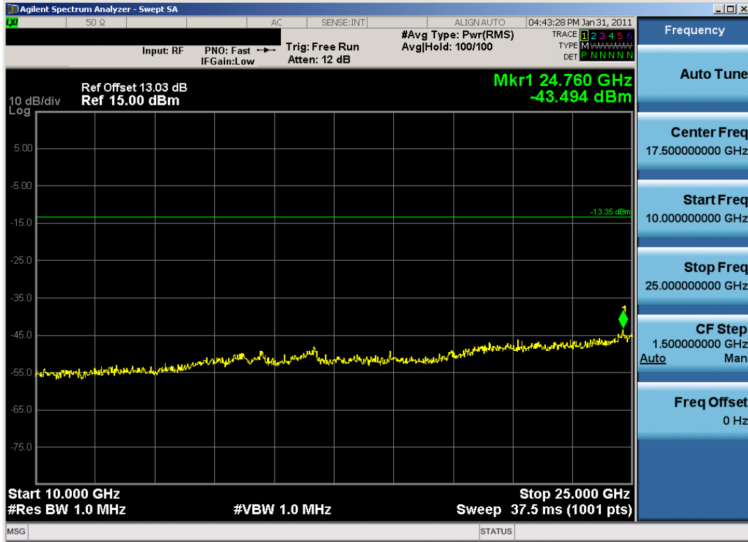
Plot 6-23. Conducted Spurious Plot (Bluetooth, 3Mbps – Ch. 78)
