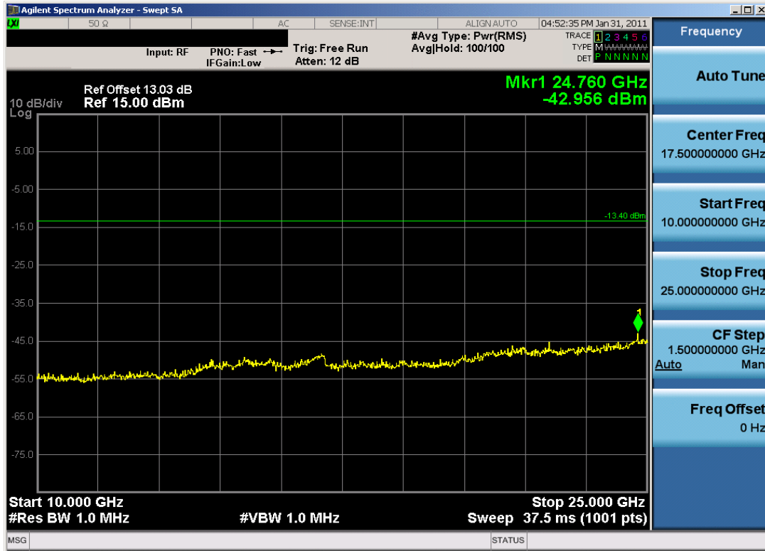
Plot 6-21. Conducted Spurious Plot (Bluetooth, 3Mbps – Ch. 39)
